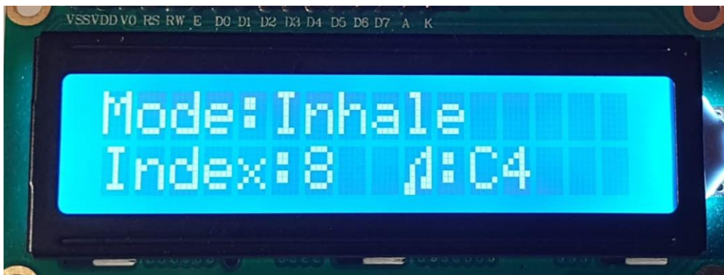
Figure 30: LCD Output: Top Left – Breath Mode, Bottom Left – Note Index, Bottom Right - Note
