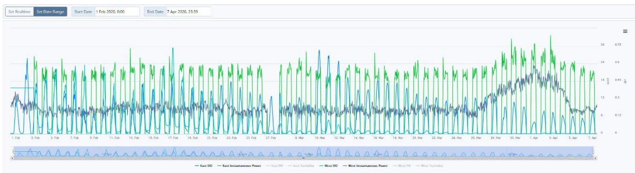
Figure 3.2.1 b Intermittent electricity supply for 12 hours for the experimental HRAP indicated by the green graph while the purple graph is the continuous power supply to the control HRAP during the Summer - Autumn season
