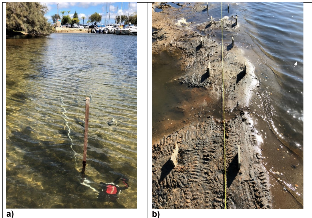
Figure 3.12 Burial of sleepers at the Swan River site: (a) commencement; and (b) completion (photographs by Trevor Winton).
