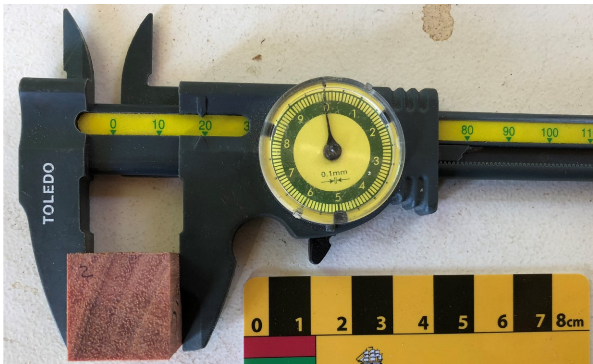
Figure 3.15 Volume measurement of timber cubes using toledo calliper (photograph by Trevor Winton).
