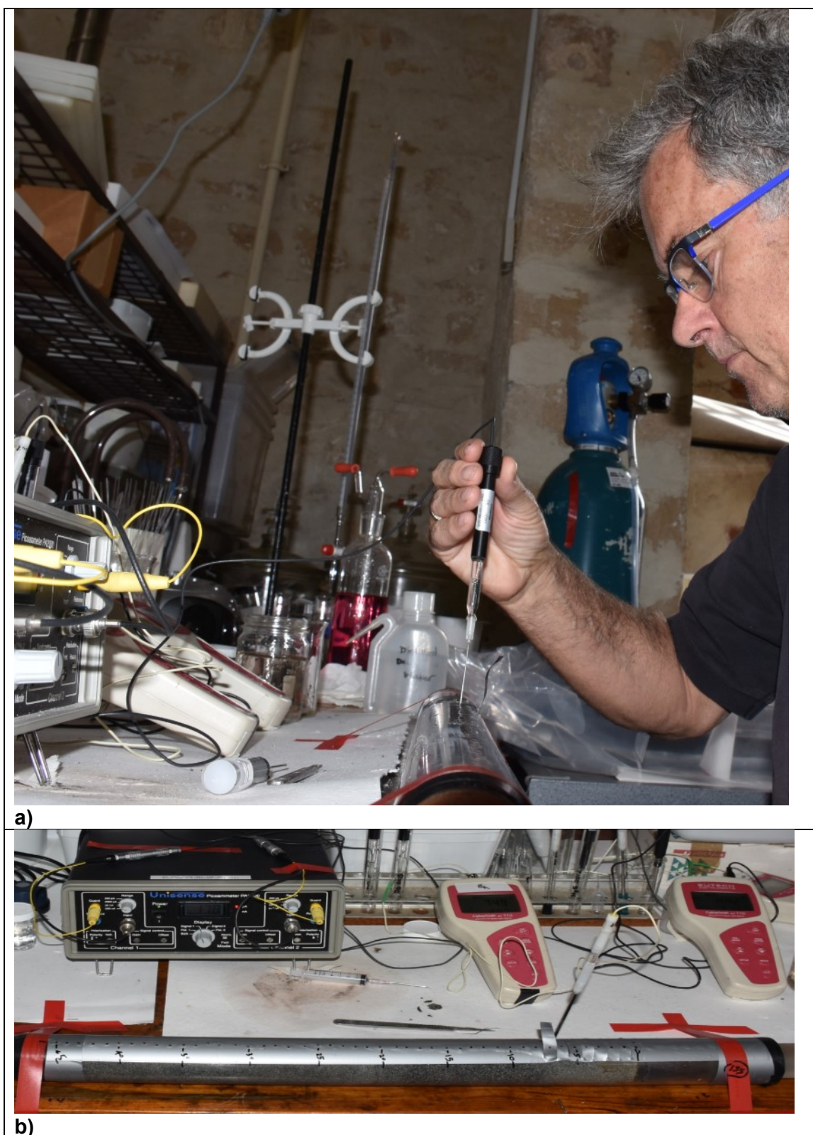
Figure 3.24 DO, Eh, pH and temperature microchemical analyses: (a) author inserting DO probe into sediment core; and (b) sediment core showing progressive uncovering and measurement within tube holes (photographs by Jon Carpenter).
