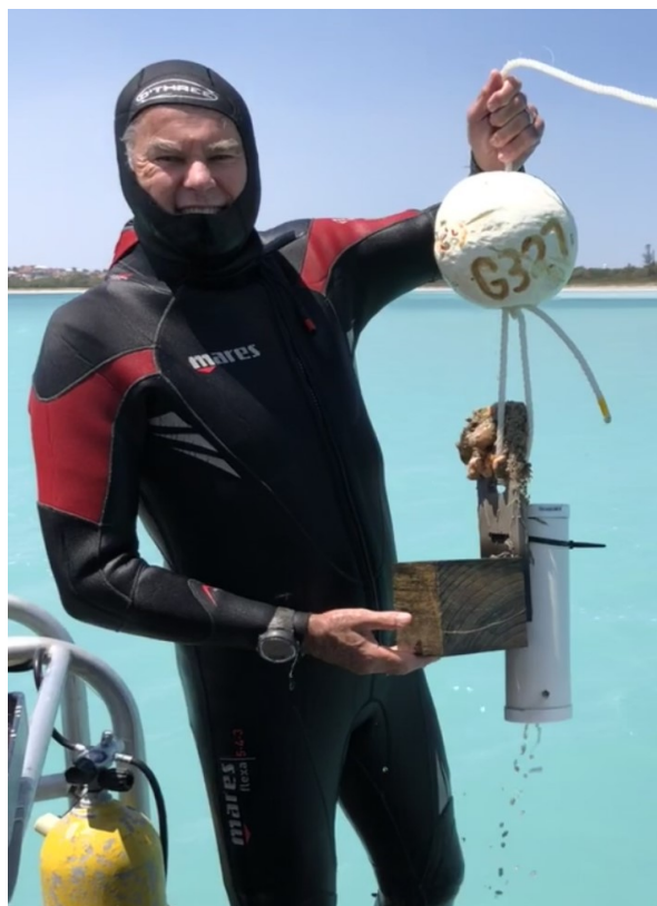
Figure 3.17 Author with recovered block Pine 10 cm DoB, James Matthews sleeper site—note attached PVC weight-tube filled with gravel (photograph by Mack McCarthy).
