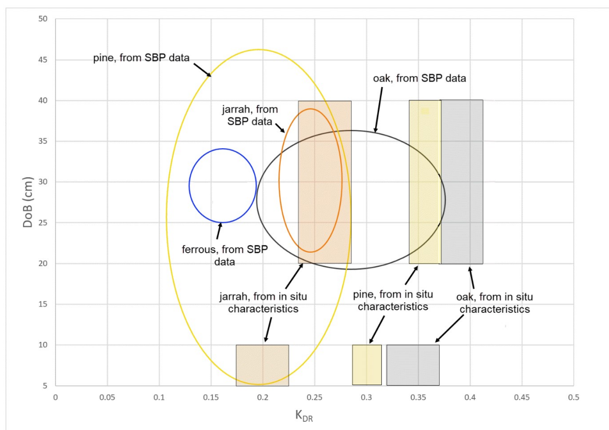
Figure 5.17 Comparison of K_{DR} values derived from SBP data and in situ characteristics.
