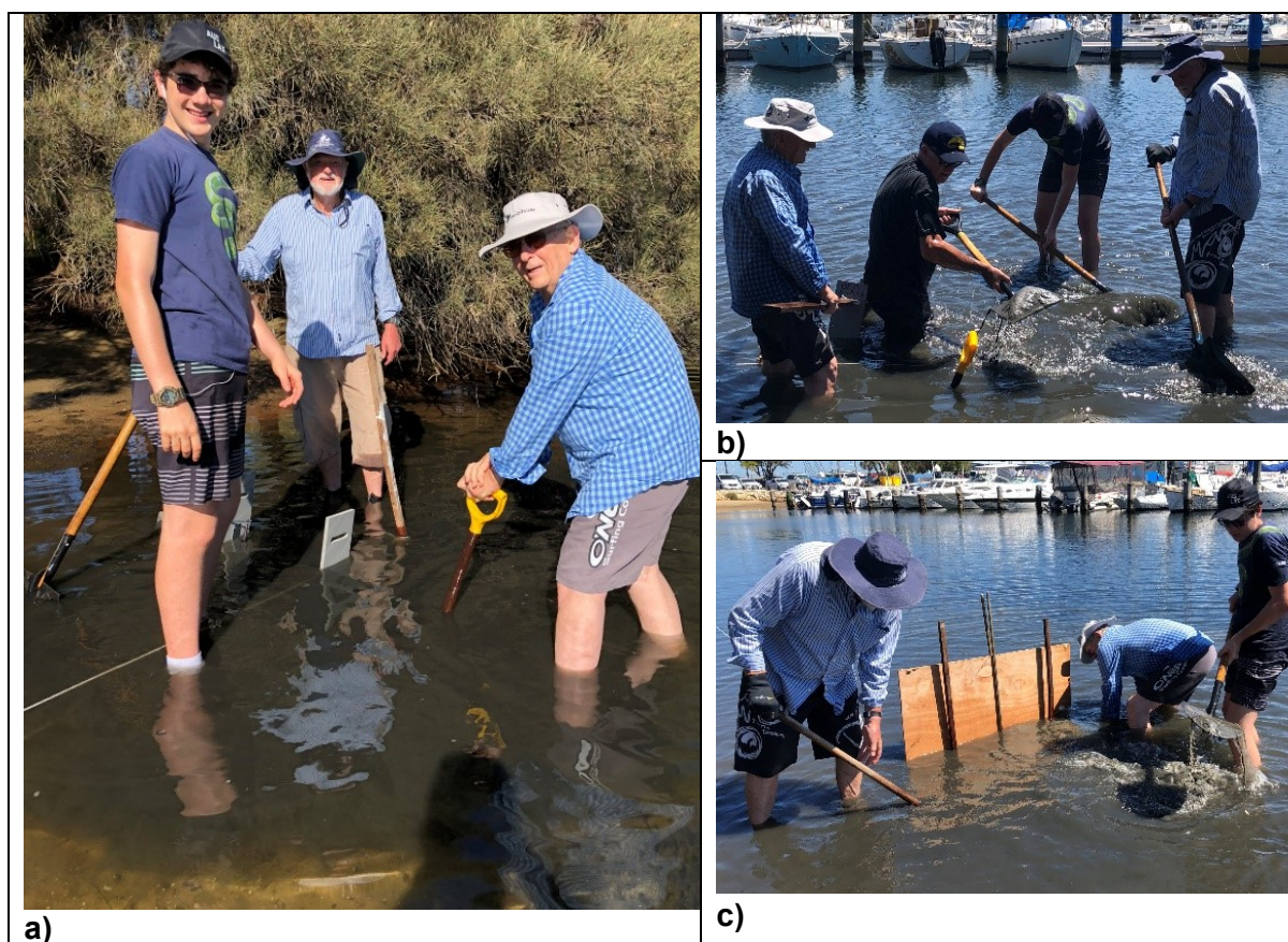
Figure 3.13 Burying of sleepers at the Swan River site: (a) MAAWA and family volunteers in shallow water; (b) burying 50 cm DoB sleepers; and (c) sheet wall to prevent sediment slumping in deep holes (photographs by Marianna Winton).
