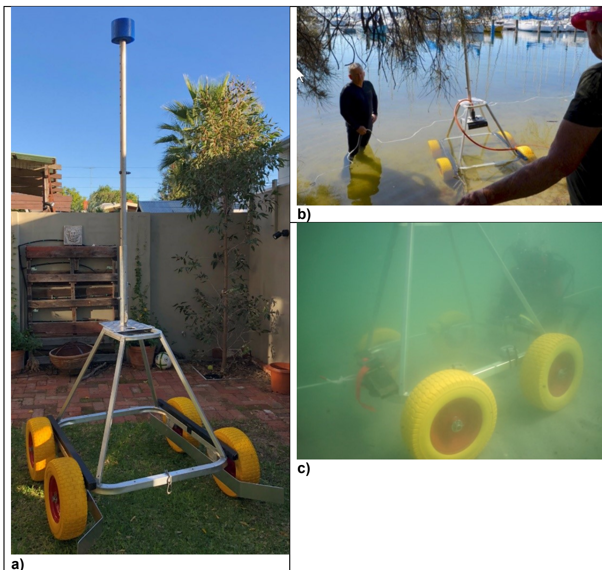
Figure 3.30 Seabed SBP sled: (a) fabricated sled and mast, without transducer and RTK rover; (b) sled entering Swan River site, showing transducer and orange dedicated power/data cable; and (c) sled on seabed at the James Matthews sleeper site (photograph (a) by Trevor Winton, (b) by Col Cochran and (c) by Ian McCann).
