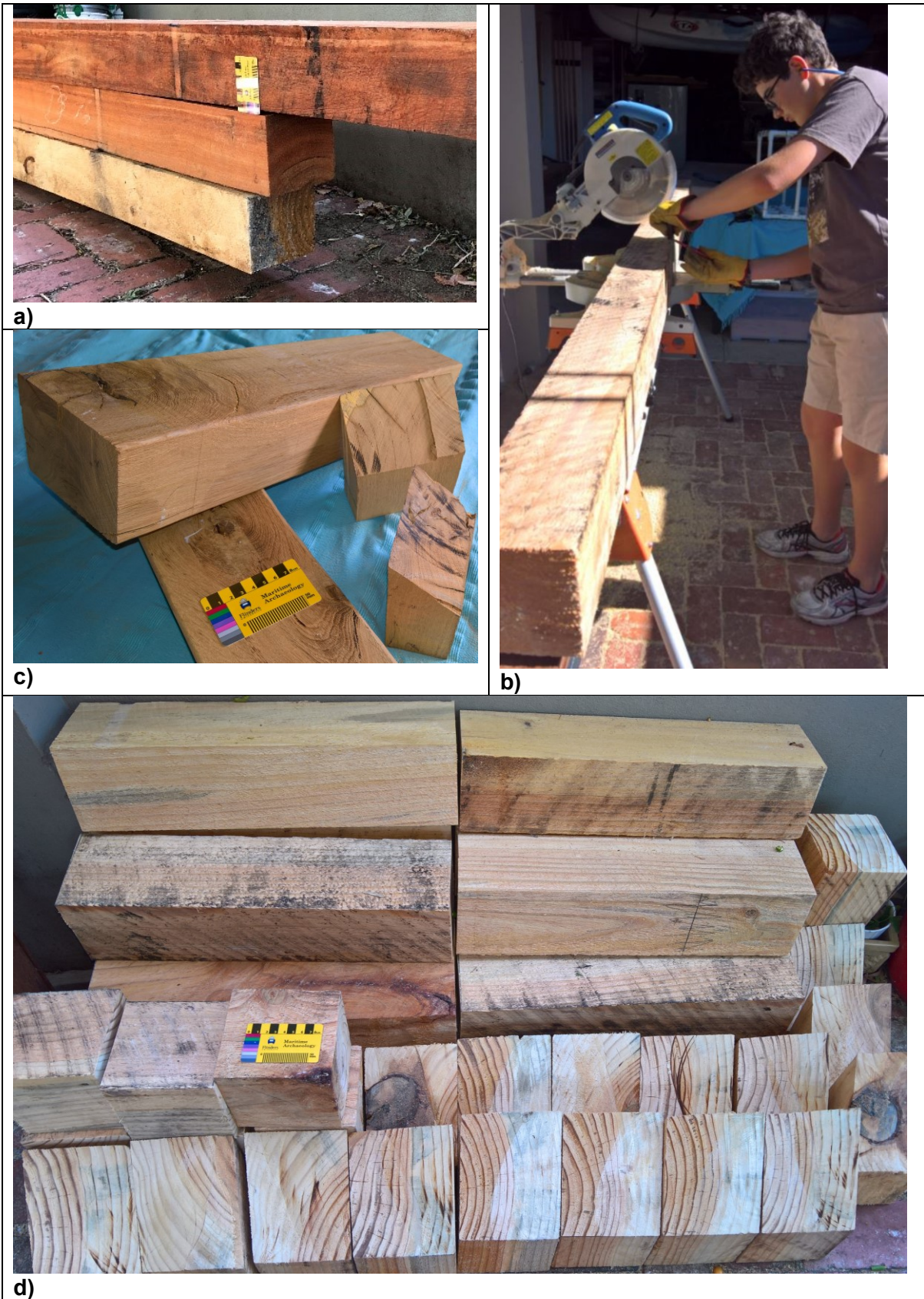
Figure 3.6 Timber sleepers and blocks: (a) lengths of freshly milled jarrah and pine; (b) cutting timbers to length; (c) oak sleepers and blocks; (d) pine sleepers and blocks (photographs by Trevor Winton).
