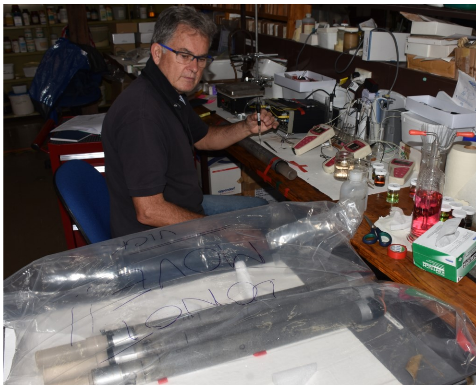
Figure 3.23 The author with sediment cores inside argon filled sealed bag and DO, Eh and pH profiling setup (photograph by Jon Carpenter).
