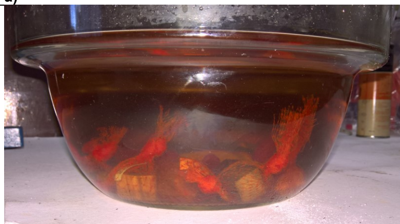
Figure 3.16 Vacuum desiccator jar with timber cubes: (a) floating; and (b) saturated (photographs by Trevor Winton).
