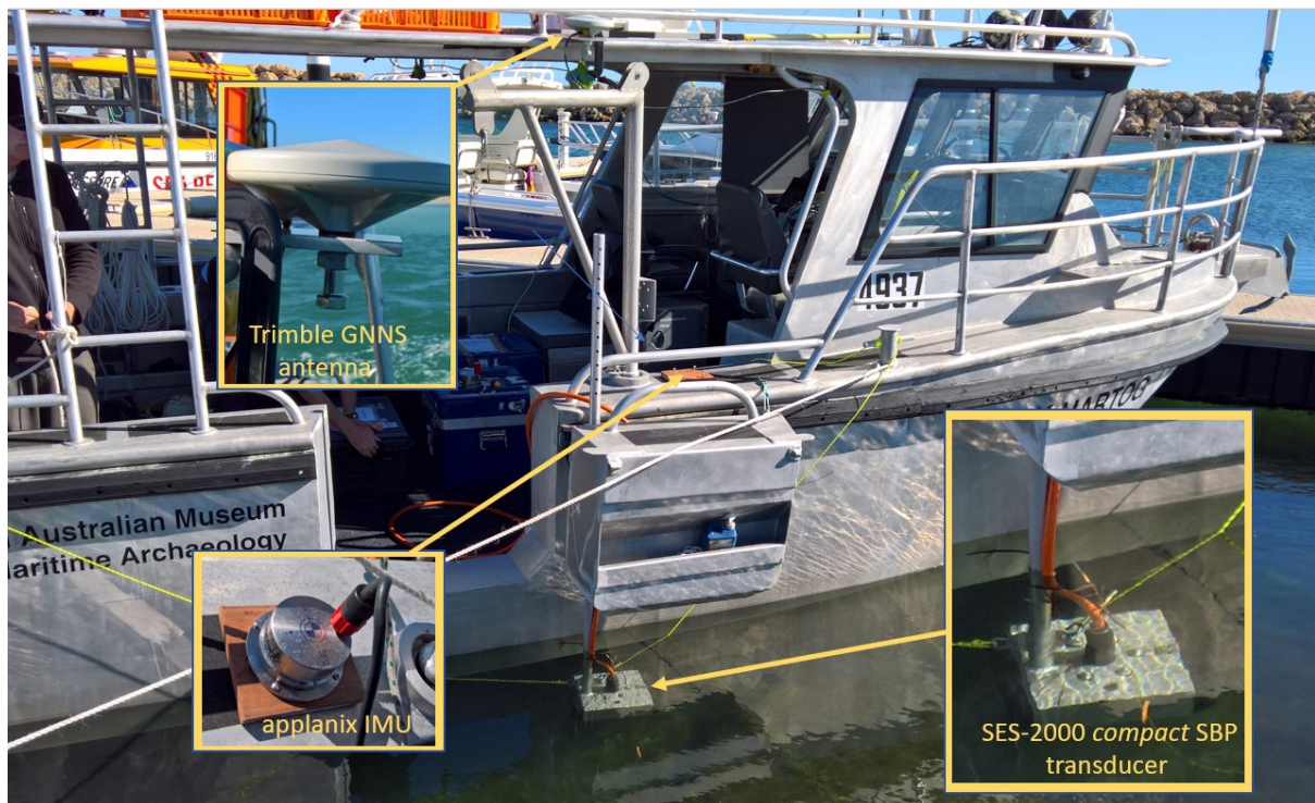
Figure 3.29 WAM research vessel Dirk Hartog showing mounting locations of SES-2000 compact SBP transducer, Trimble GNSS antenna and applanix IMU sensors (photographs by Trevor Winton).
