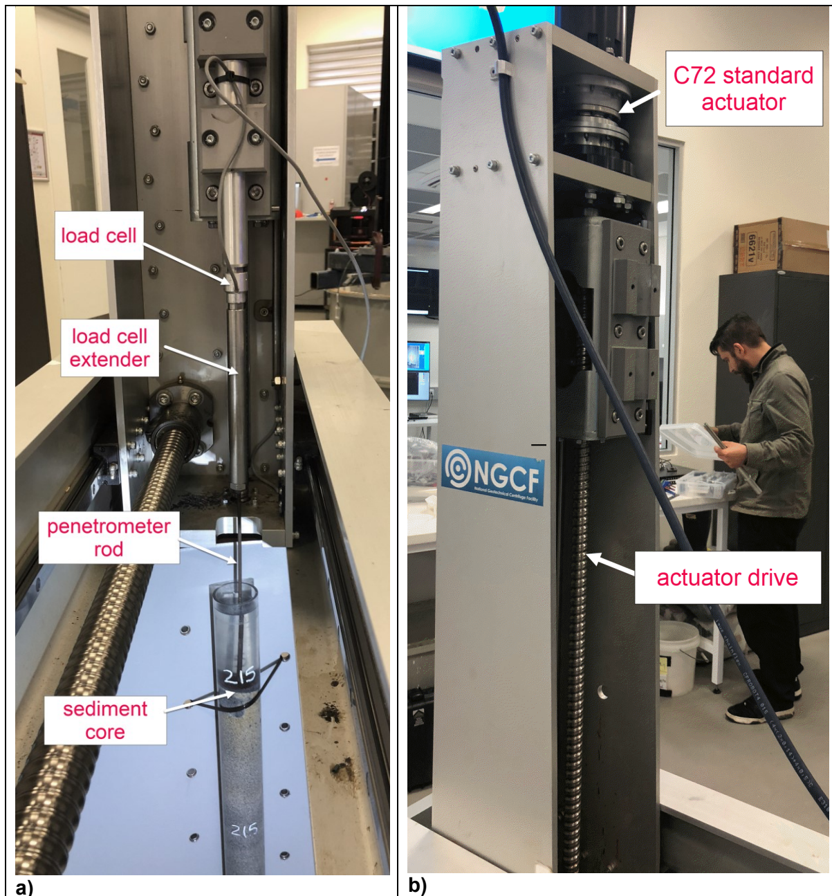
Figure 3.26 Sediment penetrometer test set up: (a) front view; and (b) side view (photographs by Trevor Winton).
