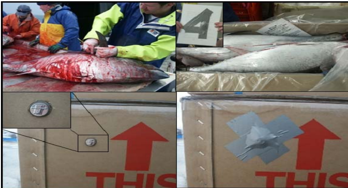
Figure 5.3: Insertion of a data logger into the post-pectoral bleed cut (top left), attachment to a laminated card for placement inside a tuna coffin (top right), and attachment and taping of a data logger to the outside of a tuna coffin in Port Lincoln, Australia (bottom two photos).
