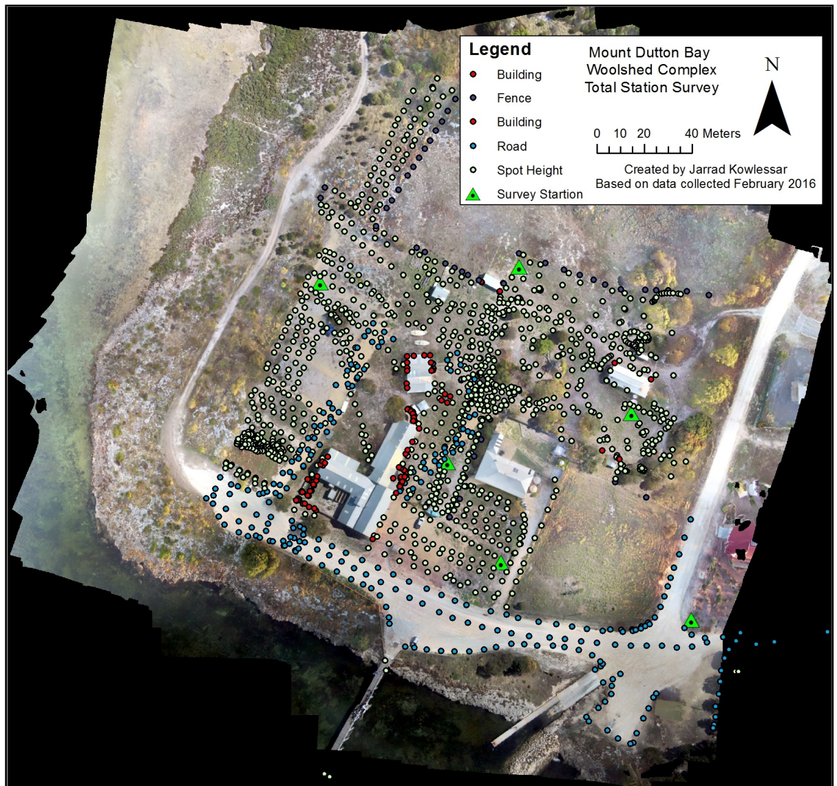
Figure 5.18: Total station survey of Mount Dutton Bay WoolShed Site
