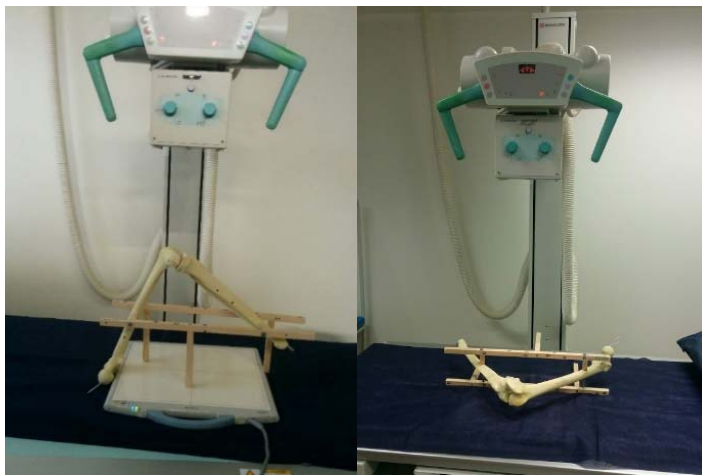
Figure 5.10. Example of AP and lateral X-ray taken for sawbone model at 90° flexion.
