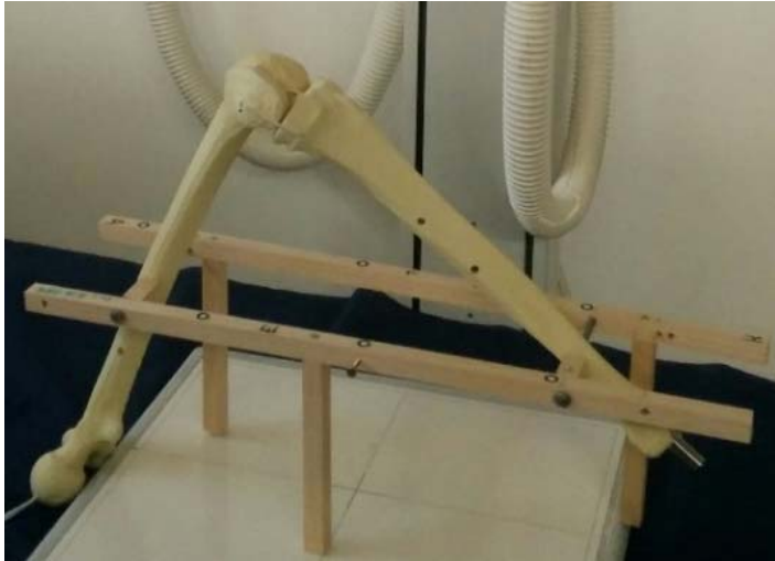
Figure 5.9. Mechanical frame constructed to hold the sawbone at different flexion angles
