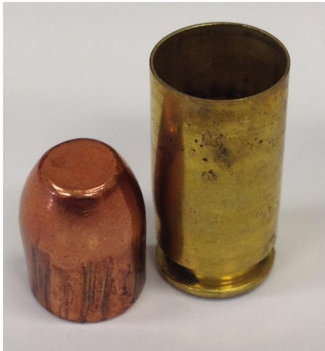
Figure 55 - Recovered fired cartridge case and projectile from 0.40 S&W Federal American Eagle Cu-TMJ, Toxic metal free primed ammunition.
