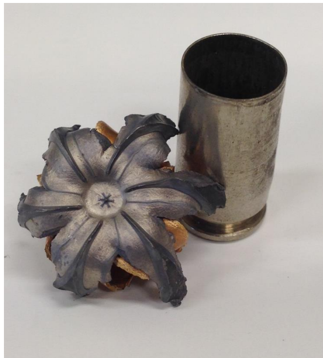
Figure 54 - Recovered cartridge case and expanded projectile from 0.40 S&W Federal Premium Law Enforcement HST ammunition. (Image supplied by author)
