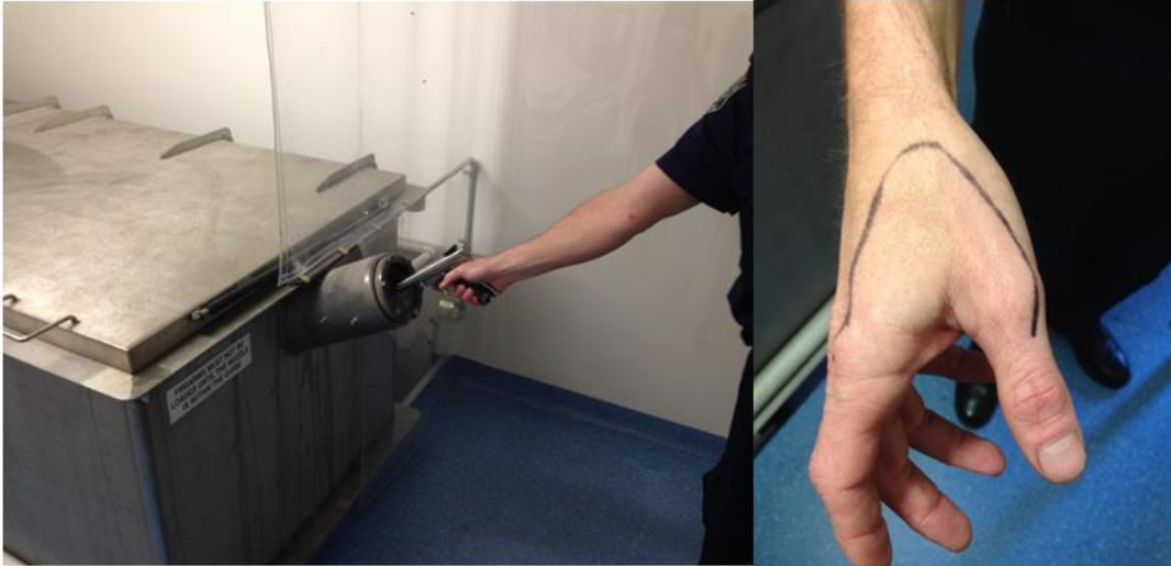
Figure 56 - Firearm discharge into bullet recovery (water) tank. (left). Area of dominant hand from which sample was collected (right).
