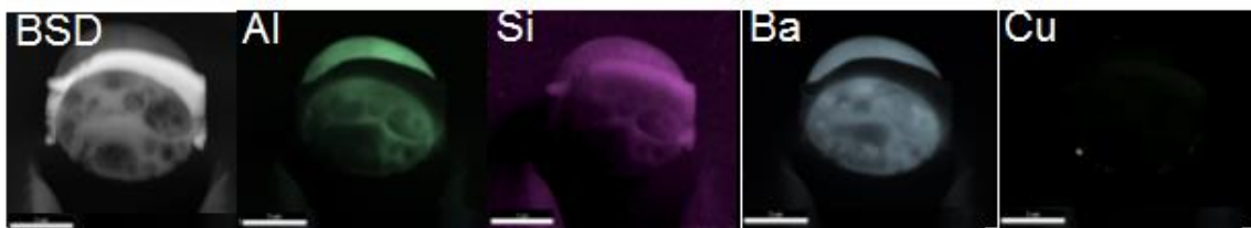
Figure 31 - Exemplar EDS spectrum of GSR from 0.40 Winchester Winclean ammunition (Inset - SE Image)
