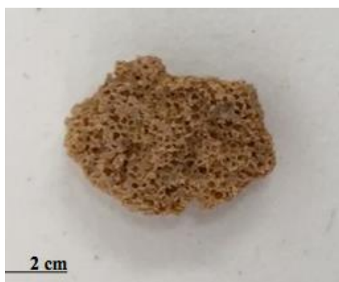
Figure 2: Image for porous polysulfide polymer This particle was isolated with a sieve with a 2.5 mm cut-off.
