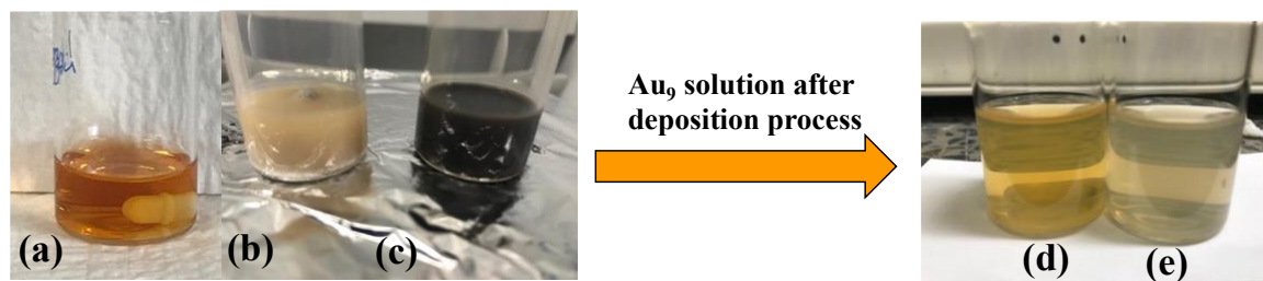
Figure 2.3. (a) Au 9 initial solution in methanol (b) white and (c) black NMTiO 2 suspension in Au 9 solution before deposition; Au 9 solution after deposition process for (d) white NMTiO 2 (e) black NMTiO 2 substrates
