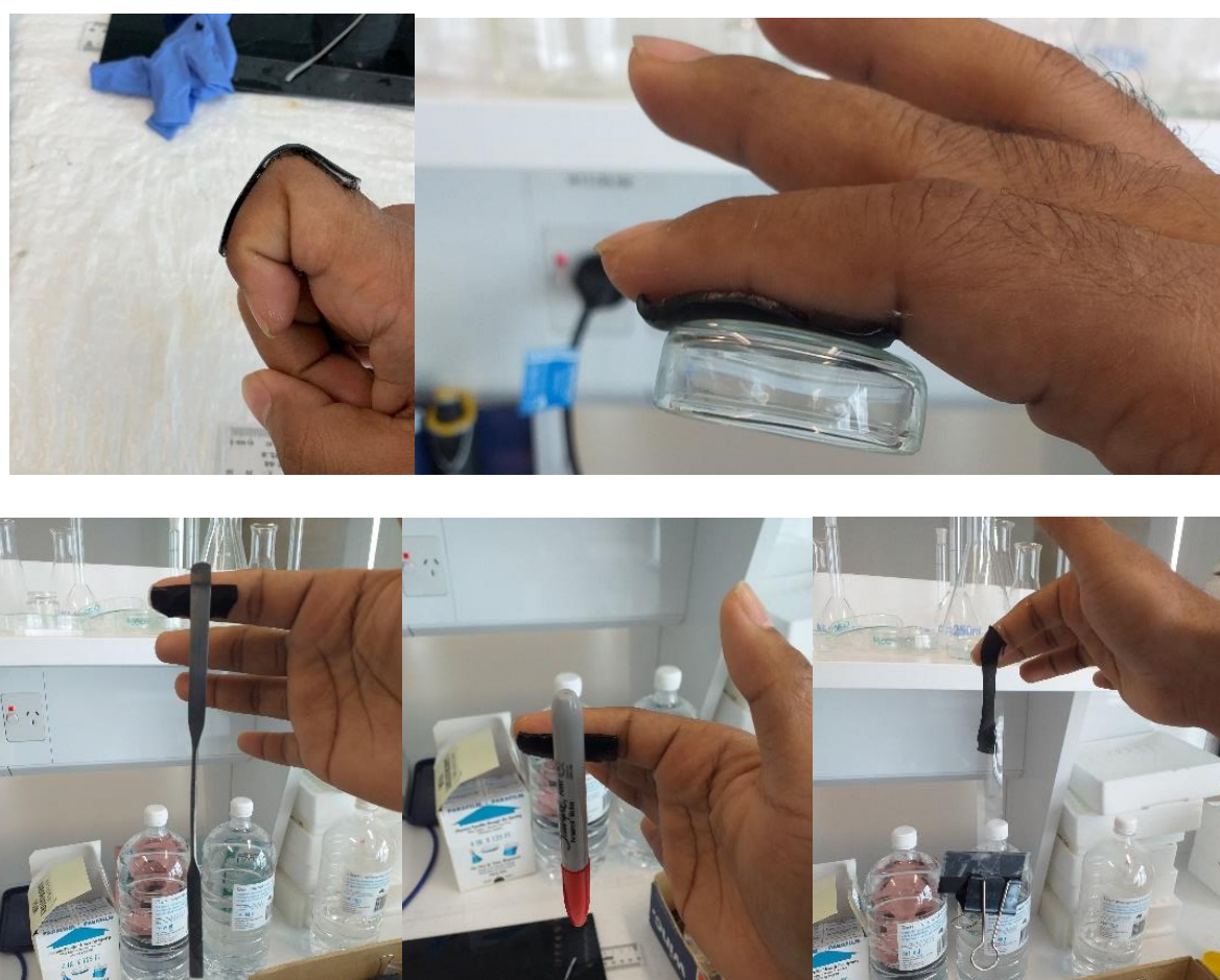
Figure 20: The demonstration of the adhesive properties on different substrates including skin, glassware, steel, and plastic
