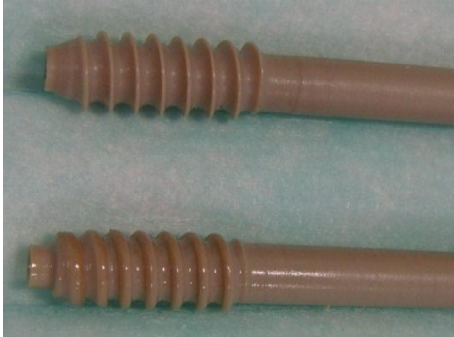
Figure 7-6: PEEK screws. The screws are shown prior to insertion (Top) and after one insertion (Bottom) into femoral head bone. The limitation of this material is evident by the shearing of the threads in the bottom screw.
