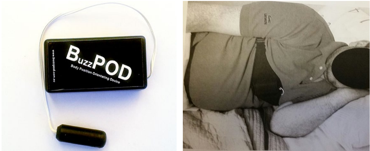
Figure 3.1 Supine-avoidance device (left) showing externalised vibration motor, and a subject wearing the device (right).
