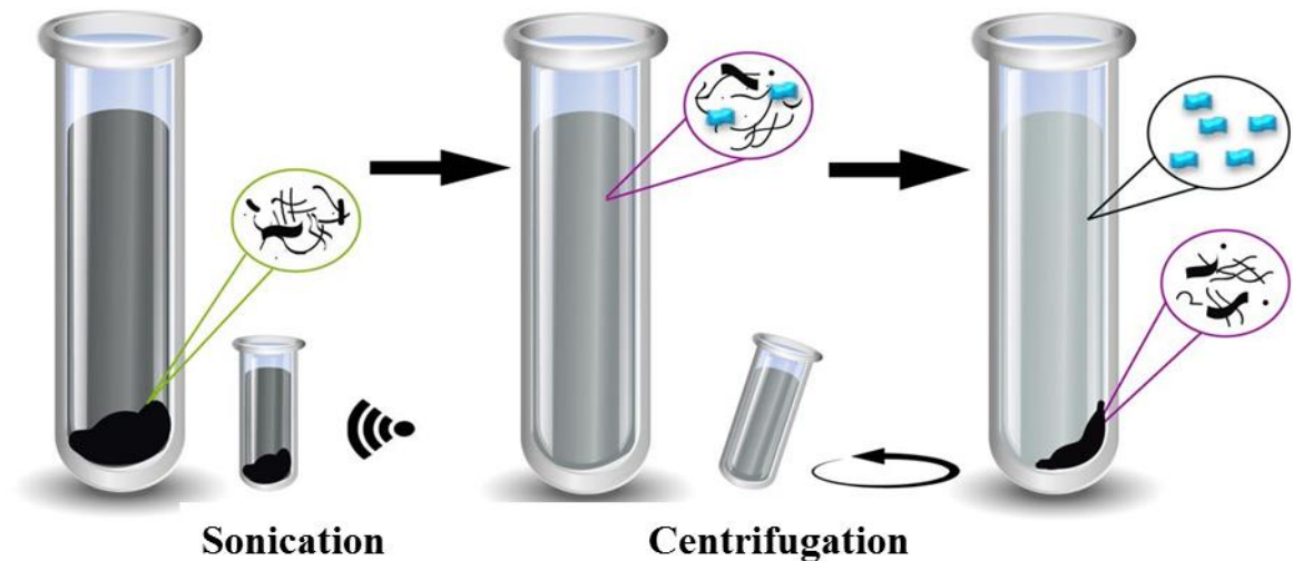
Figure 8: As-raw material of MoS 2 is dispersed in solution using sonication and centrifugation.
