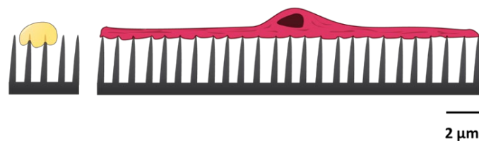
Figure 4. Schematic of bacterial cell versus mammalian cell attached to nanospikes, spreading the downward pressure experienced by the cells over a larger area, thus preventing mechanical rupture as seen in the bacterial cells-this phenomenon is known as the “bed of nails” effect.
