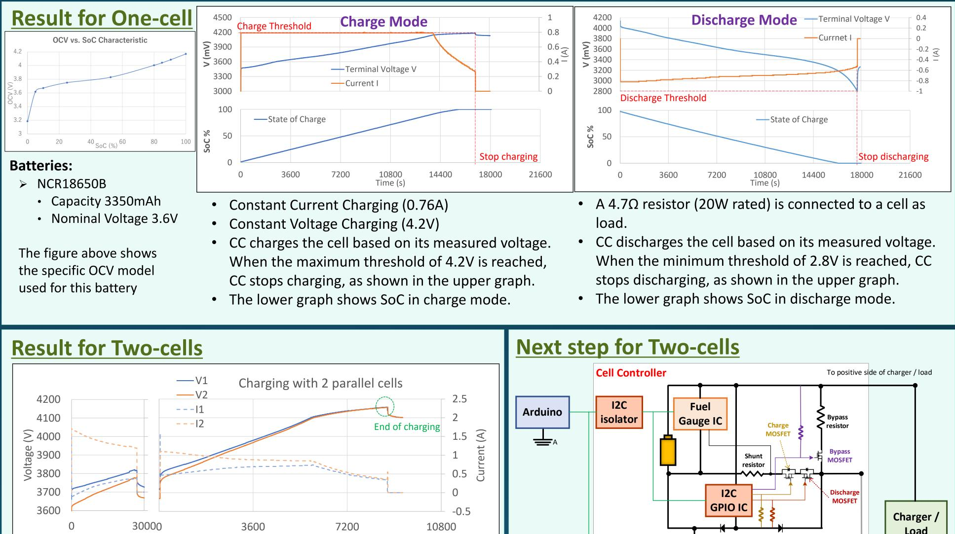
When charging two cells with different SoCs, the cell with a lower SoC is charged at a larger current than the other one.
