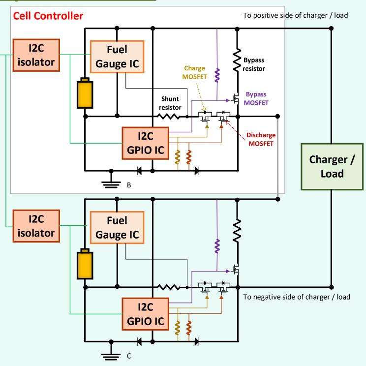
• When cells are put in series, each CC will have a different reference point (Ground).
