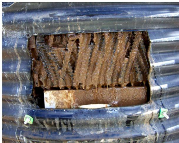
**Plate 3.18.** The original NTF: Squashed biofilm sample drawer.
