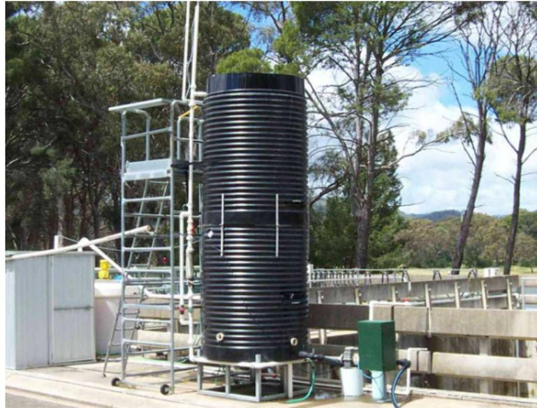
**Plate 3.15.** Earlier version of the large pilot-scale NTF.
