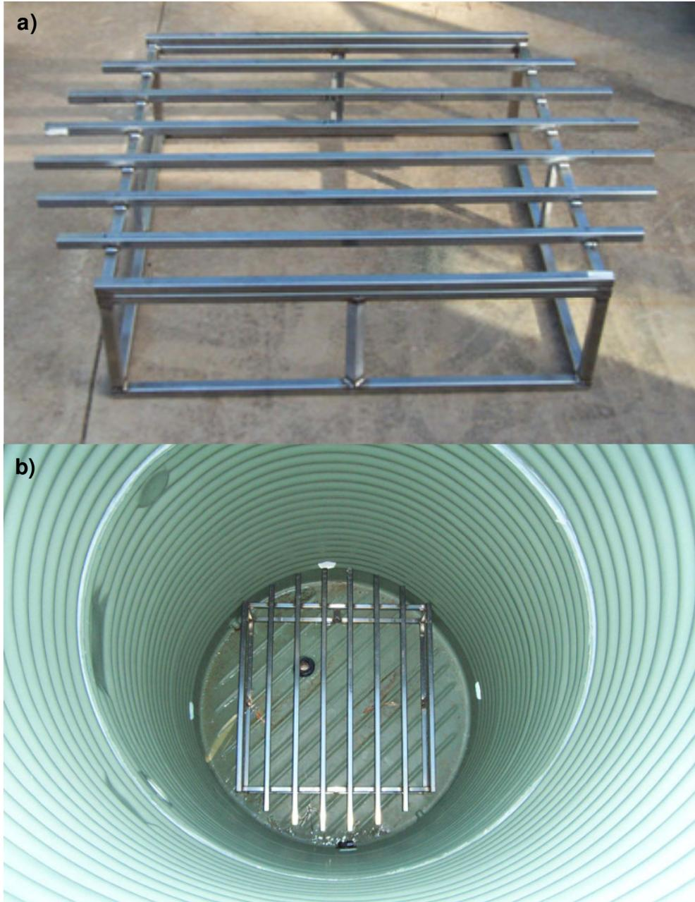
**Plate 3.3.** (a) Media support stand; and (b) birds-eye view of the stand once positioned inside the NTF column.
