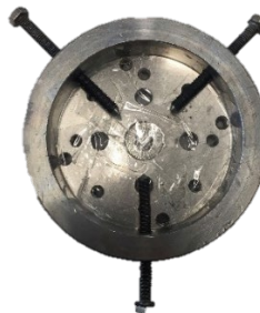
Figure B.2: Two Bolts Screws into the Cups
