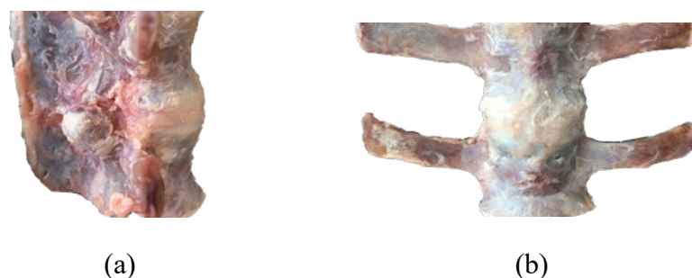
Figure 4.3: Extracted Lateral (a) and Anterior (b) Views of the L4/L5 FSU (Vertebra–Disc–Vertebra Segment) After Transversal Bisection Using a Band Saw
