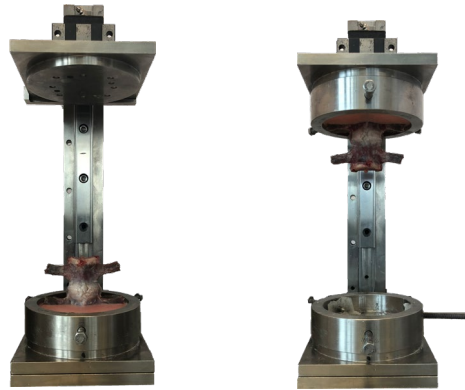
Figure B.3: Alignment Rig Used for Potting Specimen
