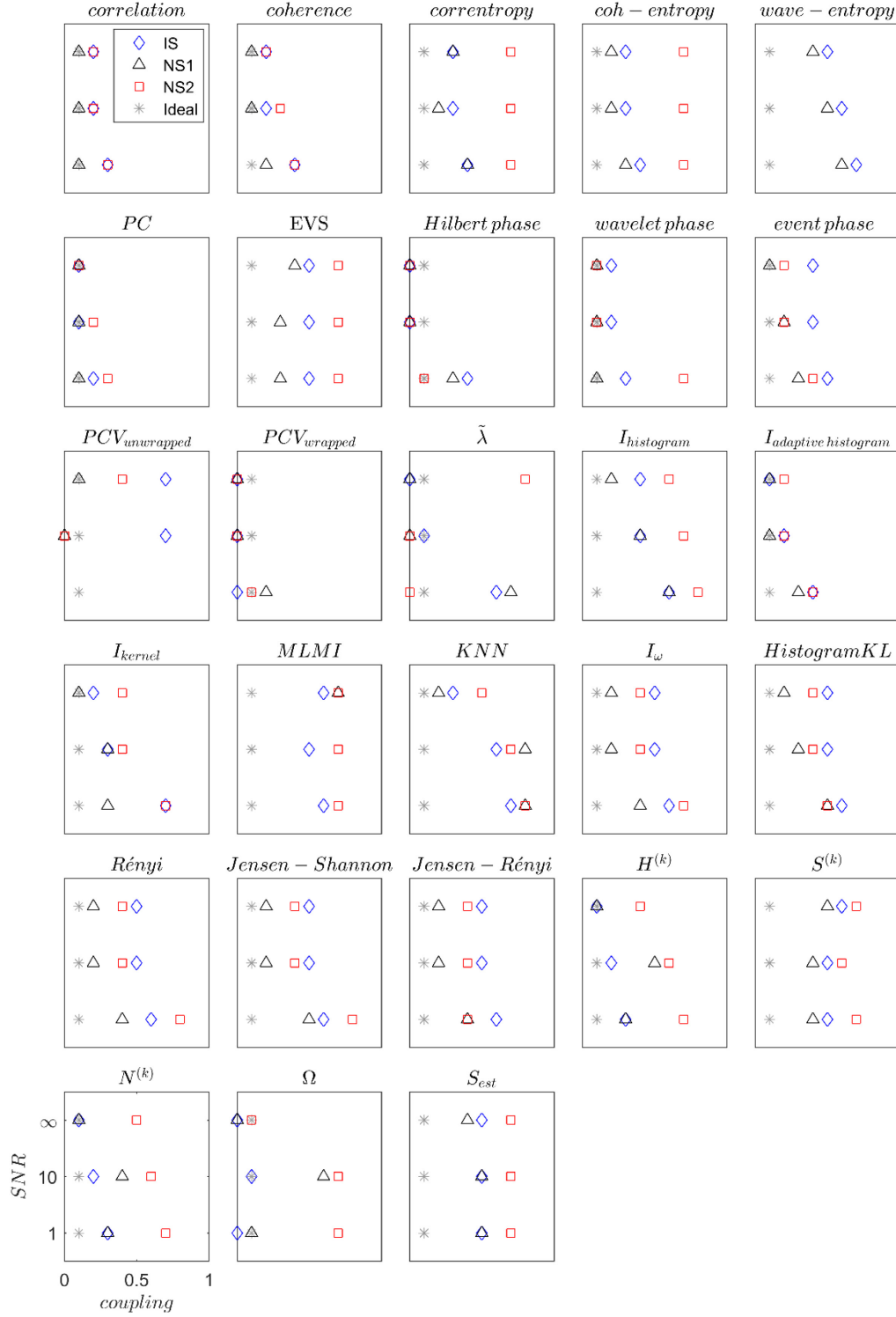
Figure 3-20: The lowest value of coupling strength that detects synchrony against SNR (noise-free, SNR of 10 dB, and SNR of 1 dB) for IS (blue diamond), NS1 (black triangle), NS2 (red square), and the ideal result (black asterisk).
