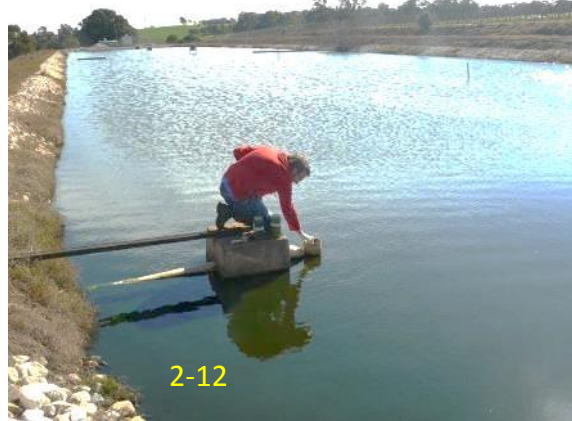
Plate 2-11 & 2-12 2-11 ISCO Avalanche refrigerated multi sampler in-situ at the KoM HRAP site and 2-12 overflow weir sample collection site at the exit point of WSP 1
