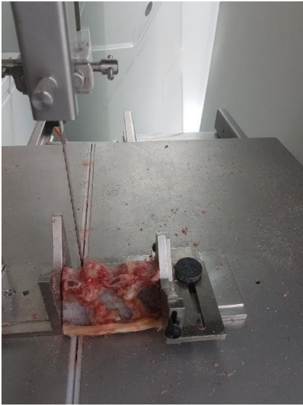
Figure 4-4 - Sheep specimen with removed soft tissues and cut at T12 L1 using a bandsaw.
