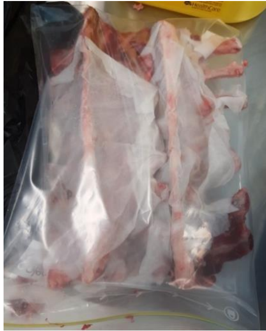
Figure 4-3 - Specimens with removed soft tissues, wrapped in paper towels, sprayed with normal saline and then zipped in plastic bags.
