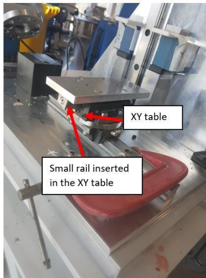
Figure 8-15: Small rail with the adaptor plate inserted into the top of XY table
