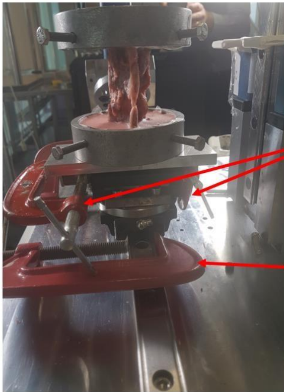
Figure 8-16: Picture displaying the clamps that stop the sliding motion of the cups therefore stopping them from falling off the rails.
