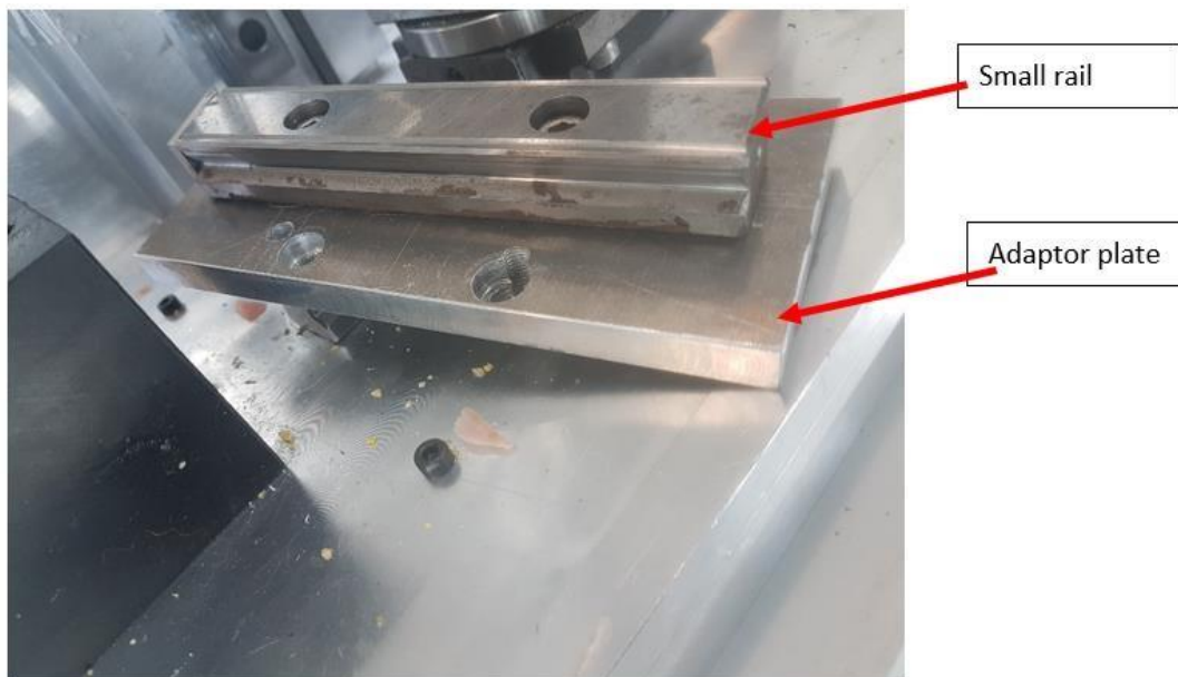
Figure 8-11: This picture indicates the adaptor plate attached on the small rail.
