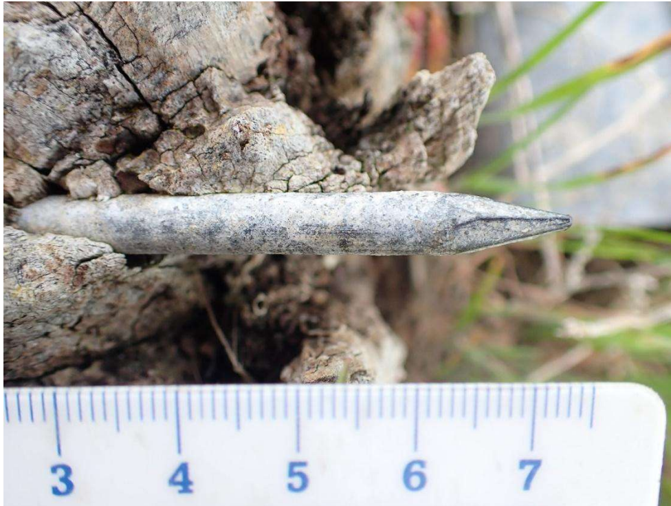
Figure 34: Galvanised spike/nail approximately 150mm in length (1mm scale divisions).
