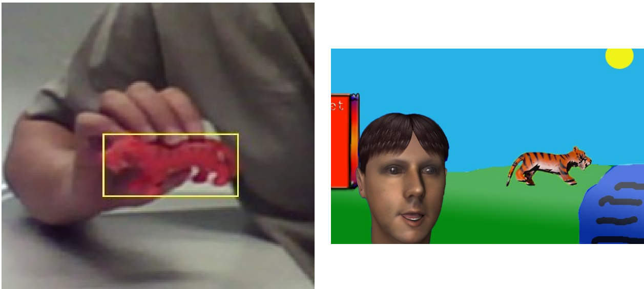
Figure 8.4: The view of the tiger from the webcam. Note that the camera is looking from the front, so the virtual image seems reversed. Spot the Tiger heads for the lake in the virtual world, movements controlled by the actions depicted in the picture on the left.
