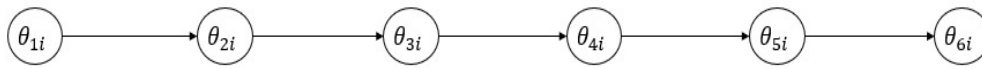
Figure 6.25 A simple DAG which represents the dependency between the levels \theta_{ci} in Model 2 of the Bayesian Networks Modelling
