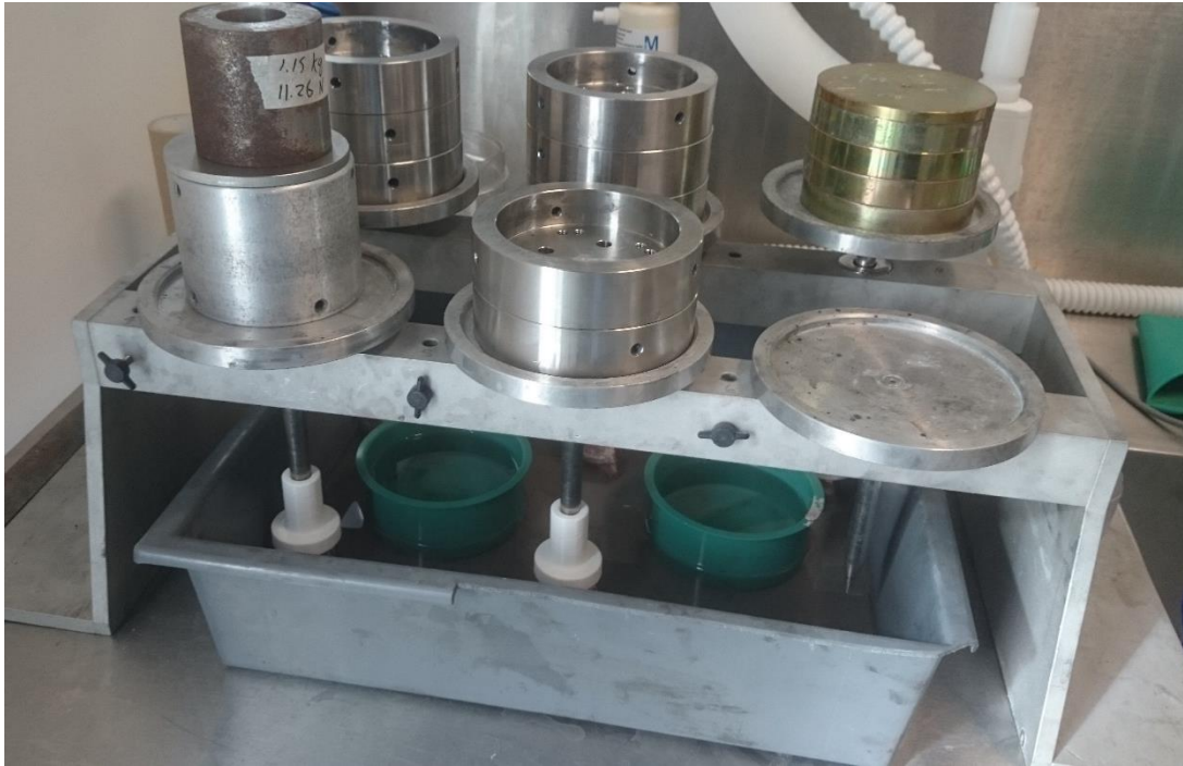
Figure 5-3, Specimens hydrating in PBS under load
