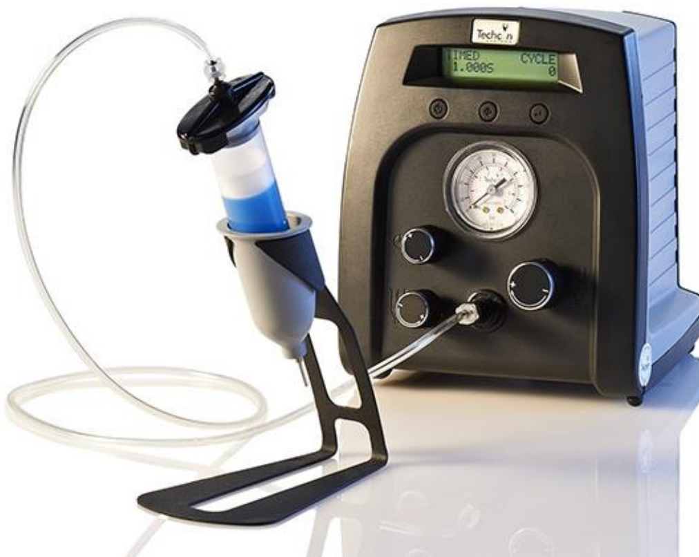
Figure 4-2, Techcon TS250 Pneumatic Paste dispenser (“Digital Fluid Dispenser - TS250,” n.d.)
