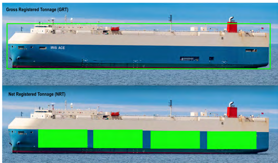
Figure 5 Ship GRT (Top) versus NRT (Bottom) (Adapted from "IRIS ACE [IMO: 9515474] is a Vehicles Carrier with 43709 gross tonnage..." by Rab Lawrence). CC BY 2.0
