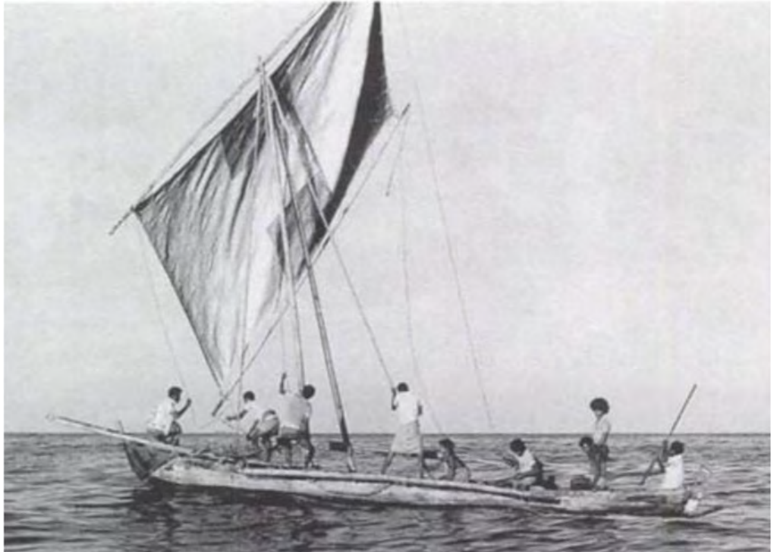
Figure 45 Bipod-masted Solorese coastal whaling boat (Reproduced with permission PLSclear. Barnes 1996:202).
