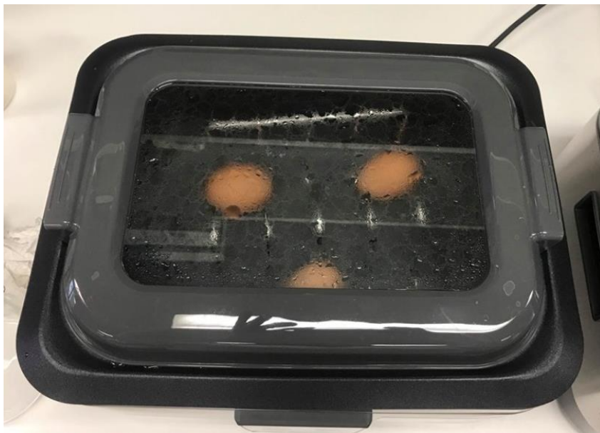
Figure 3.8: Eggs immersed in a commercial sous-vide water bath at 57°C to decontaminate the eggshell artificially contaminated with Salmonella
