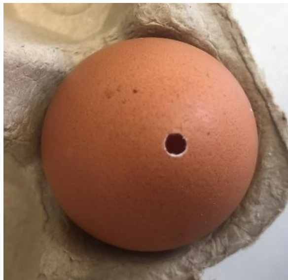
Figure 3.3: Eggs were drilled to insert the temperature rod of the HOBO temperature logger to observe the internal temperature changes during treatment in the sous-vide water bath at 57°C
