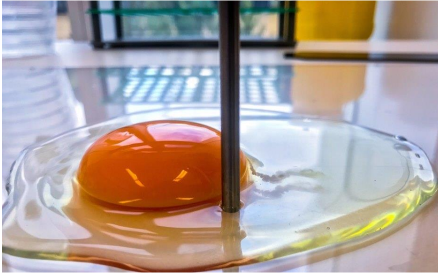
Figure 3.16: The height of the egg albumen was measured using a micrometer to calculate the Haugh unit to determine the quality of the egg following the heat treatments
