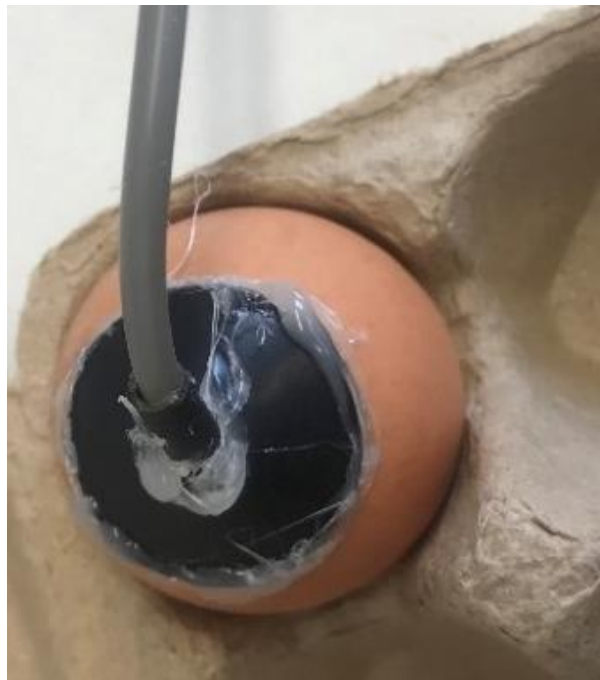
Figure 3.4: The egg sealed with hot, quick drying glue after placing the thermistor into the egg prior to placing the eggs with the thermistor in the sous-vide water bath
