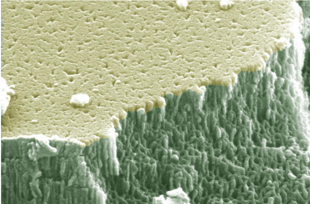
**Figure 1.3 - SEM of a partially broken pSi film revealing an array of straight pores.**
