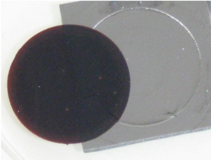
**Figure 1.6 – An intact freestanding pSi film liberated from the silicon substrate by electropolishing.**
