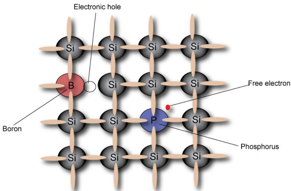
**Figure 1.4 – An illustration for both boron (p-type) and phosphorous (n-type) doping within the silicon lattice. Boron doped silicon contains electronic holes that can act as current carriers. The current carriers for phosphorous doped silicon are the free surplus electrons.**
