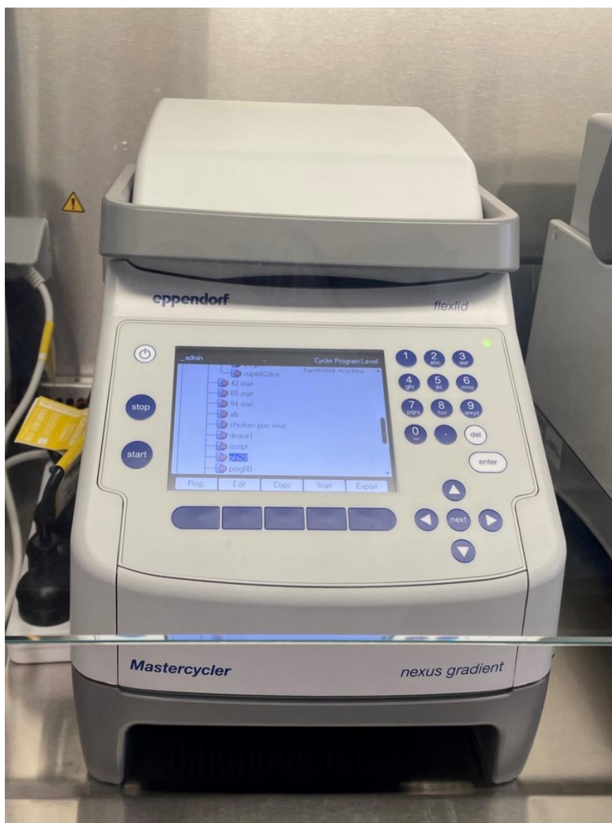
Figure 14. Eppendorf Mastercycler Nexus Gradient PCR machine. it used for the amplification of DNA from the skin microbiome of elasmobranchs. This instrument was essential for both PCR amplification and cleaning PCR products, offering flexibility in setting temperature gradients and time periods for each stage of the PCR cycle, ensuring accurate and reliable results during genetic analysis of the isolated microbes.
