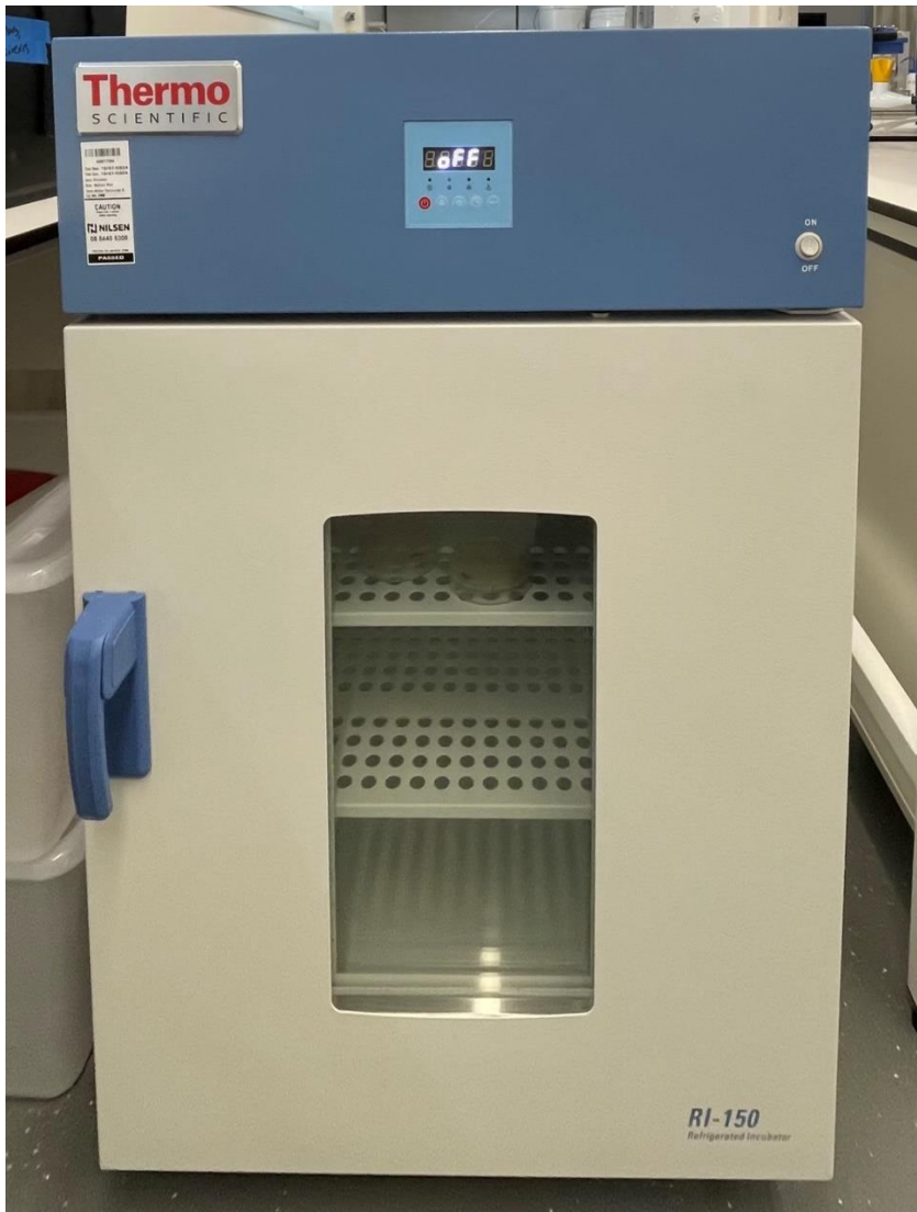
Figure 13. ThermoFisher Scientific RI-150. This refrigerated incubator used for growing isolated bacteria from elasmobranchs. This incubator maintained a constant temperature of 18°C, ensuring optimal conditions for marine microbial growth during the disc diffusion assays for antibiotic sensitivity testing.
