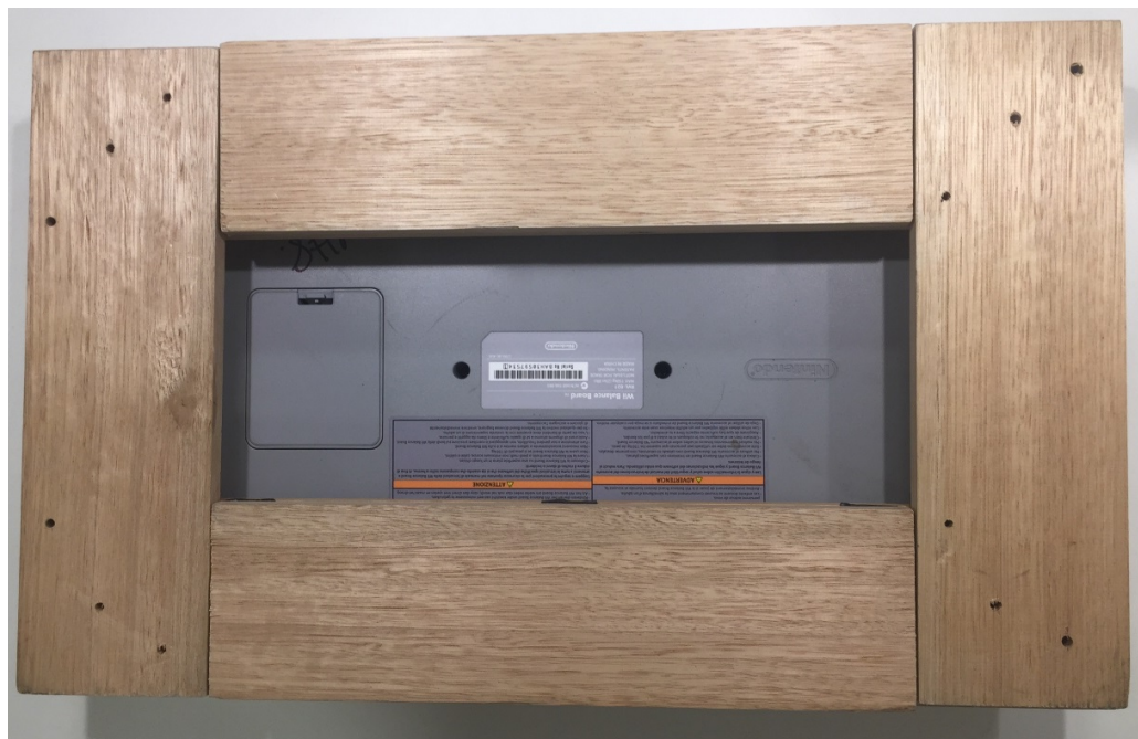
Figure 22: Back view of the mounting frame used to attach the Wii Balance Board to the leg press machine
