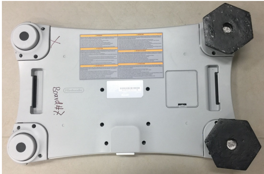
Figure 14: 4kg are placed on the left sensors of the Wii Balance Board
