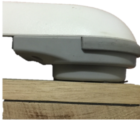
Figure 21: View of the Wii Balance sensor attached to the mounting frame
