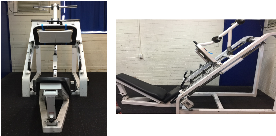
Figure 19: Left: front view of the Wii Balance Board mounted on the leg press machine. Right: side view of the Wii Balance Board mounted on the leg press machine.
