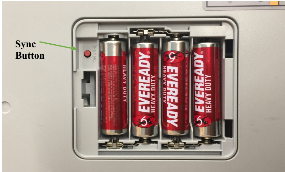
Figure 9: Sync button must be pressed in order to connect the Wii Balance Board with the Arduino
