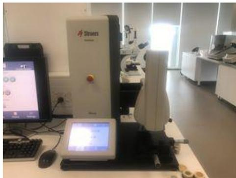
*Figure 10 – Struers's Vickers hardness tester.*
