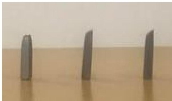
*Figure 21 - Comparison of fracture positions for dissimilar weld samples. Pristine sample (left) argon heat treated (centre) and air heat treated (right).*
