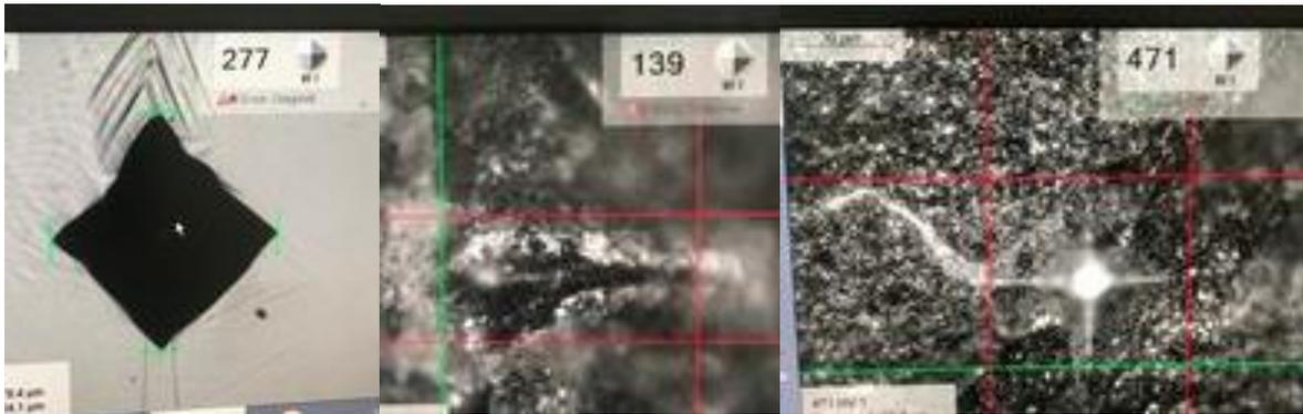
*Figure 38 - Example of slipping in multiple situations, Polished samples (left) PCM heat treated samples (centre) Unpolished samples (right).*
