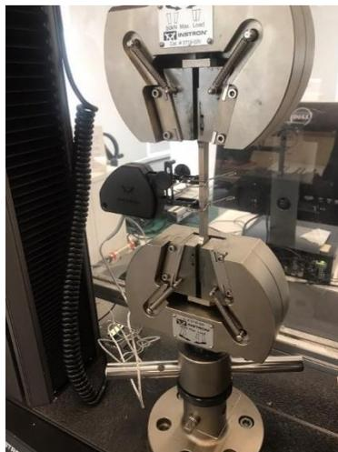
*Figure 9 – Instron stress tester.*
