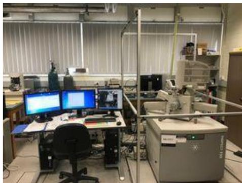
*Figure 13 – Scanning electron microscope accompanied by energy dispersive X-ray spectroscopy.*
