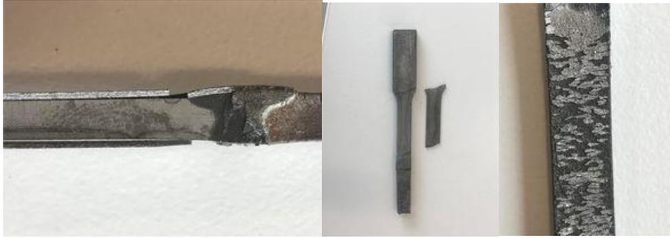
*Figure 32 – PCM heat treated dissimilar weld sample after fracture. Inconel 625 to weld cross section (left). Coving plate broken away from Inconel 625 (centre). Flaking of stainless steel 316L (right).*
