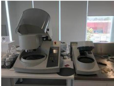
*Figure 6 – Struers's polishing and grinding machine.*
