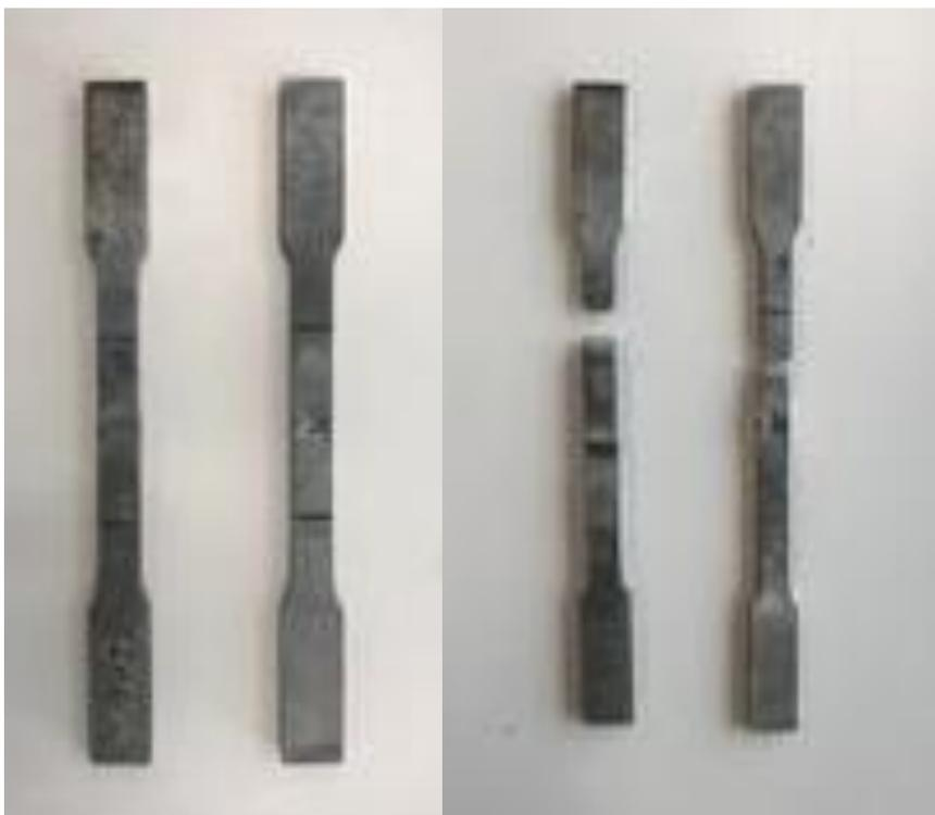
*Figure 35 - PCM heat treated dogbone samples both before (left) and after (right) fracture.*
