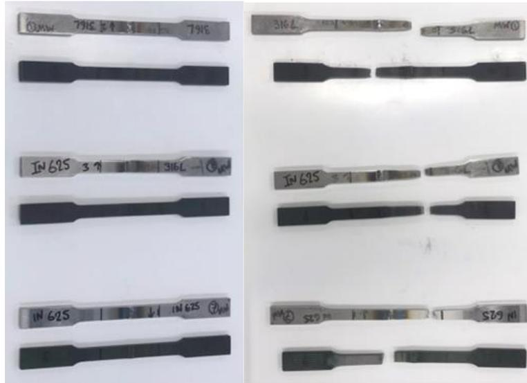
Figure 29 – Pristine and argon heat treated dogbone samples, before (left) and after (right) the tensile strength test.
