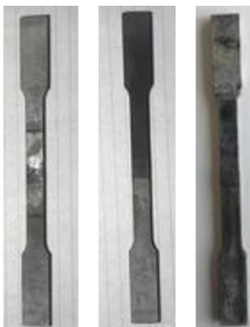
*Figure 31 – PCM heat treated dogbone samples. Dissimilar weld front (left) and back (centre), accompanied with front image of stainless steel 316L similar sample (right).*
