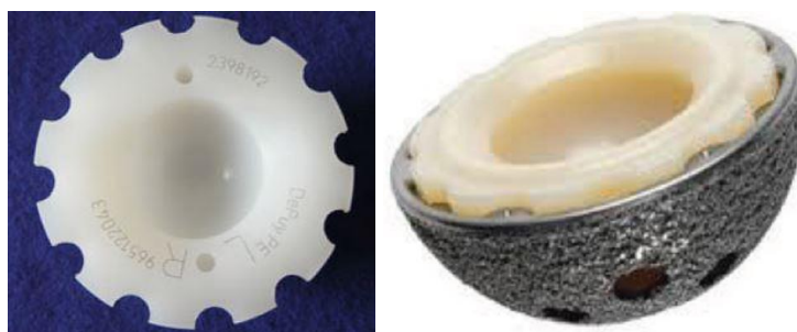
Figure 2.8 A Charnley polyethylene cemented cup (Wroblewski et al., 2016) and a titanium cementless cup with a polyethylene liner (Knight et al., 2011)
