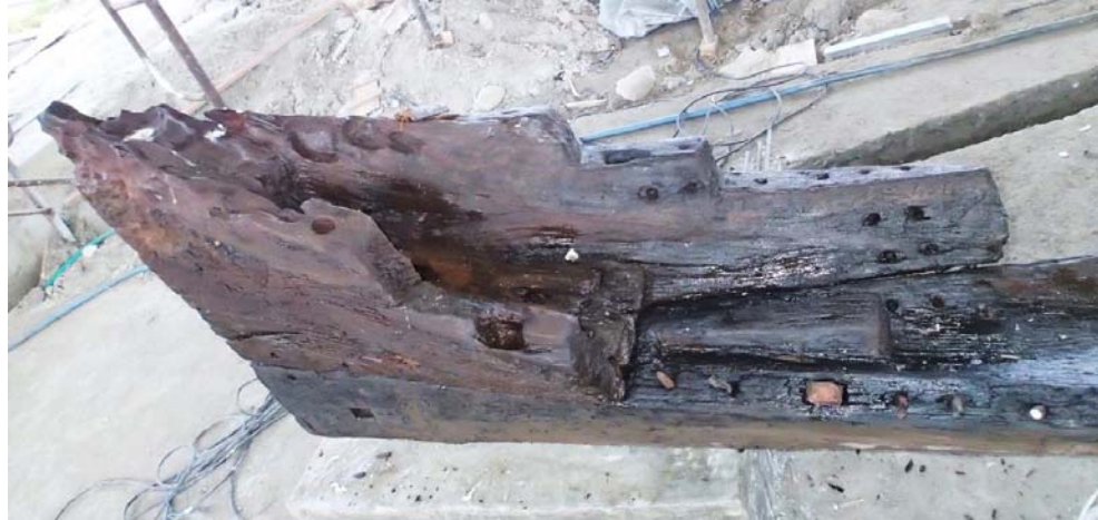
Figure 4.9. The wing-end on the bow of the Punjulharjo boat which sits on top of the keel plank (Photograph by author, 29 December 2017).
