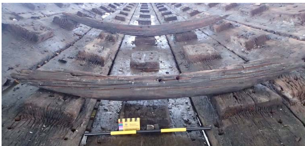
Figure 4.13. Two pieces of floor timber of the frame (Photograph by author, 30 December 2017).
