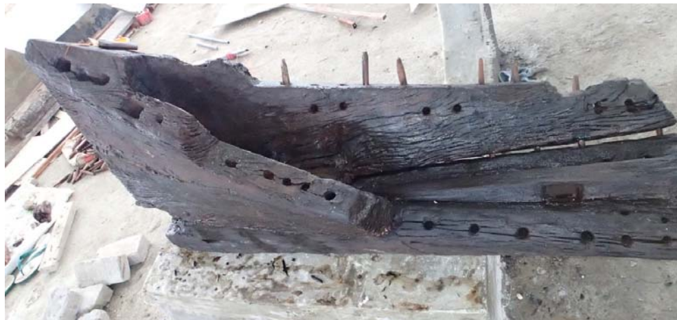
Figure 4.10. The wing-end on the stern of the Punjulharjo boat shows the three types of fastening used; dowel, mortise-tenon, and lashing (Photograph by author, 29 December 2017).
