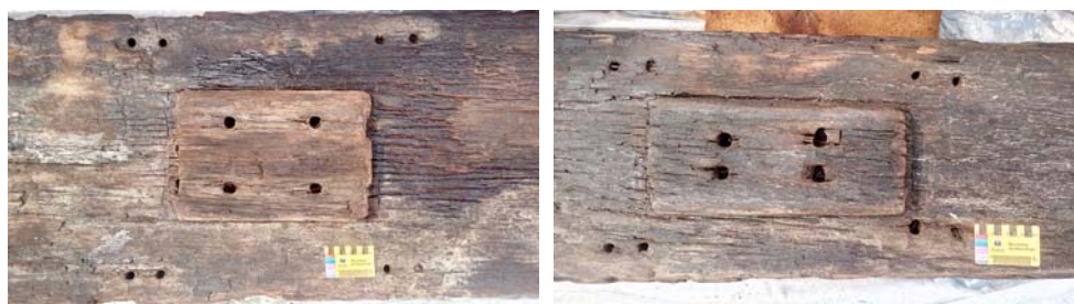
Figure 4.5. Different size and shape between the lug on the amidship (left) and towards the end (right) on the keel plank (Photograph by the author, 11 November 2017).
