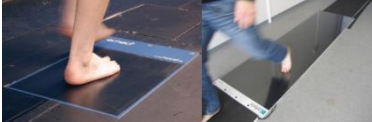
Figure 2.3: Examples of platform-based foot plantar pressure sensor plate. (Abdul Razak et al. 2012)
