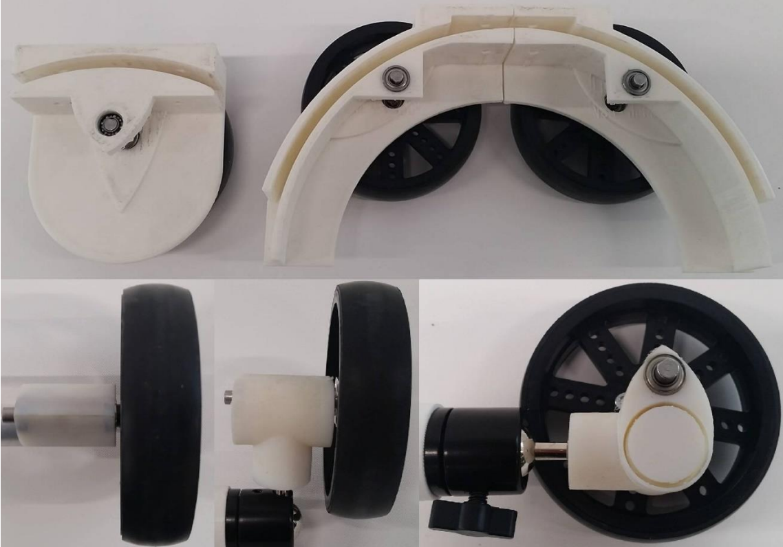
Figure 5.9: 3D printed wheel mounts with the wheels, bearings and the drive shaft installed.
