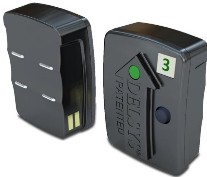
Figure 2.6: Delsys wireless Trigno EMG sensor system. (Delsys 2016)
