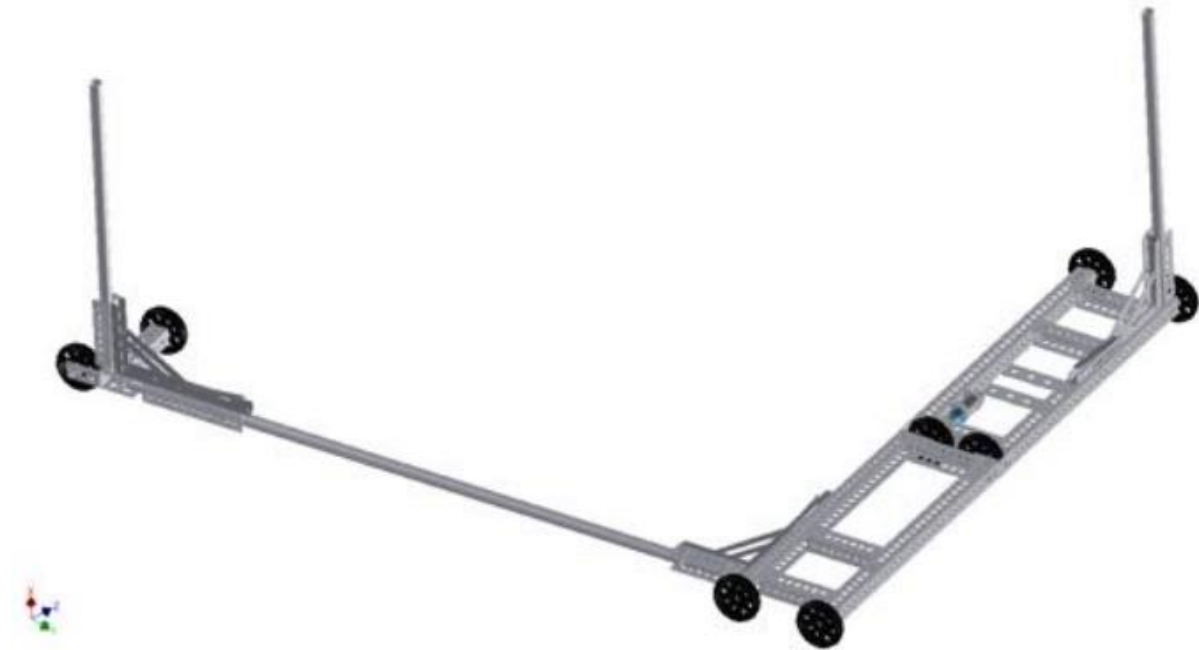
Figure 4.1: GaitScanner CAD assembly of previous structural design
