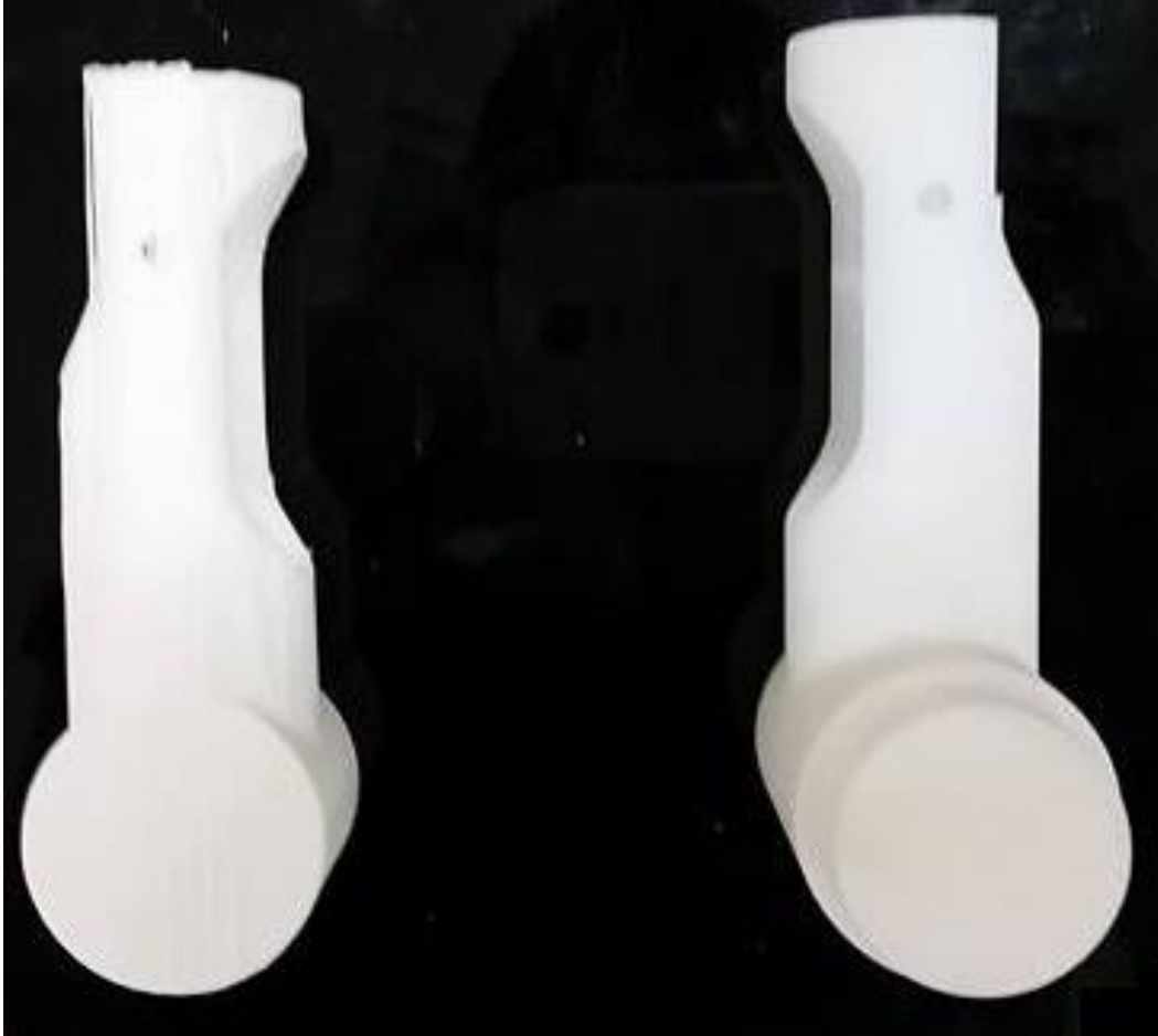
Figure 5.6: Comparison of 3D printing: MakerBot Replicator 2 (left) and Stratasys Connex 260 (right).
