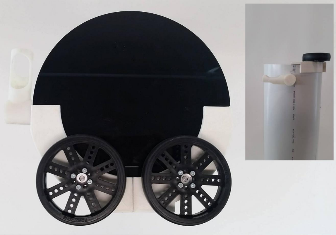
Figure 5.10: 3D printed wheel mounts with the wheels connected to the edge of the pipe.
