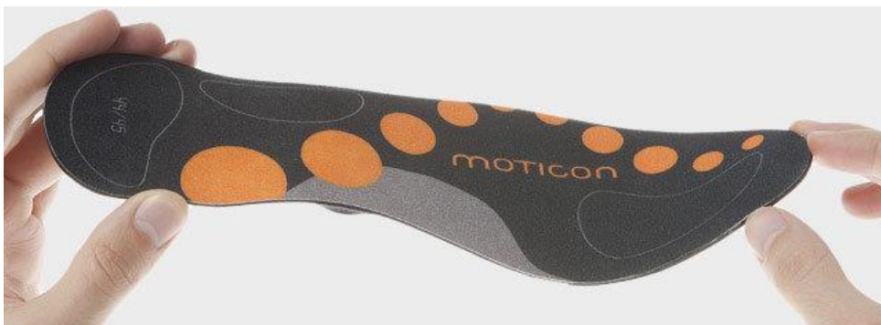
Figure 2.4: Moticon OpenGo insole measurement device. (Moticon 2016)
