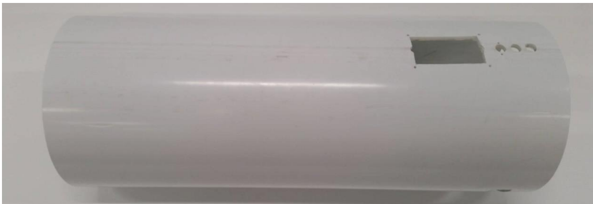
Figure 5.3: PVC pipe cut to specified dimensions.
