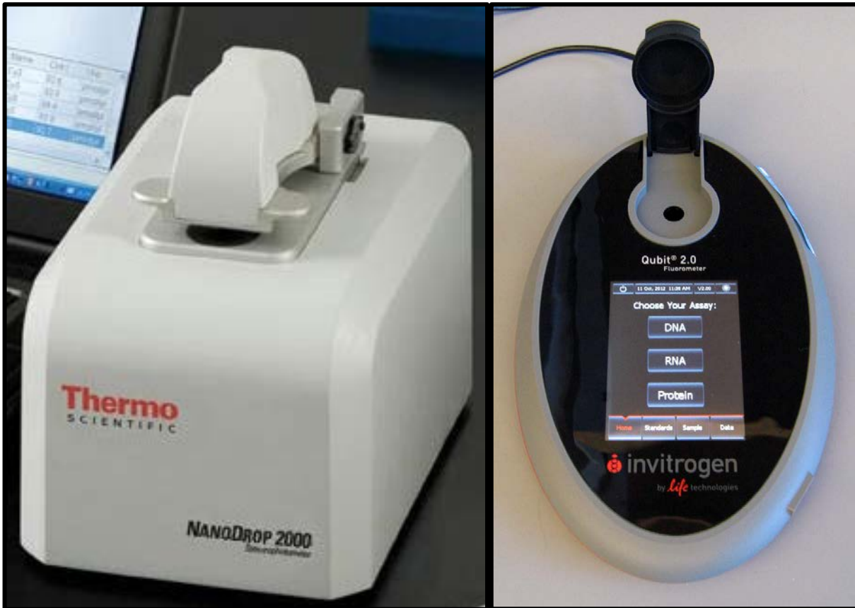
Figure 1.3 – A bench top UV spectrophotometer (left) and a newer style Qubit® 2.0 Fluorometer (right).
