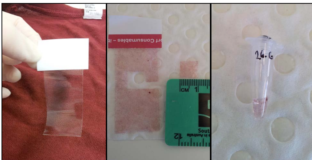
Figure 6a.7 – Tape lifting item A1, central piece of tape cut for direct PCR, and cut tape inside a 0.2 mL PCR tube.
