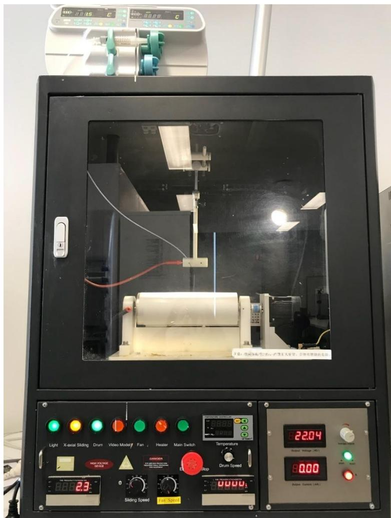
Figure 10 – NEU-Pro Electrospinning Unit
