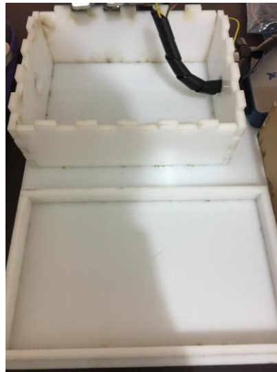
FIGURE 63: LASER CUT FABRICATED CASING FOR ULTRASOUND DAQ SYSTEM
