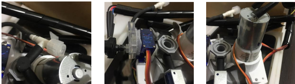
FIGURE 53: TUBING, PRESSURE CHAMBER AND LEAK VALVE
