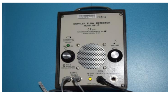
FIGURE 23: ULTRASONIC BLOOD FLOW METER BY PARKS MEDICAL ELECTRONICS MODEL 811-B
