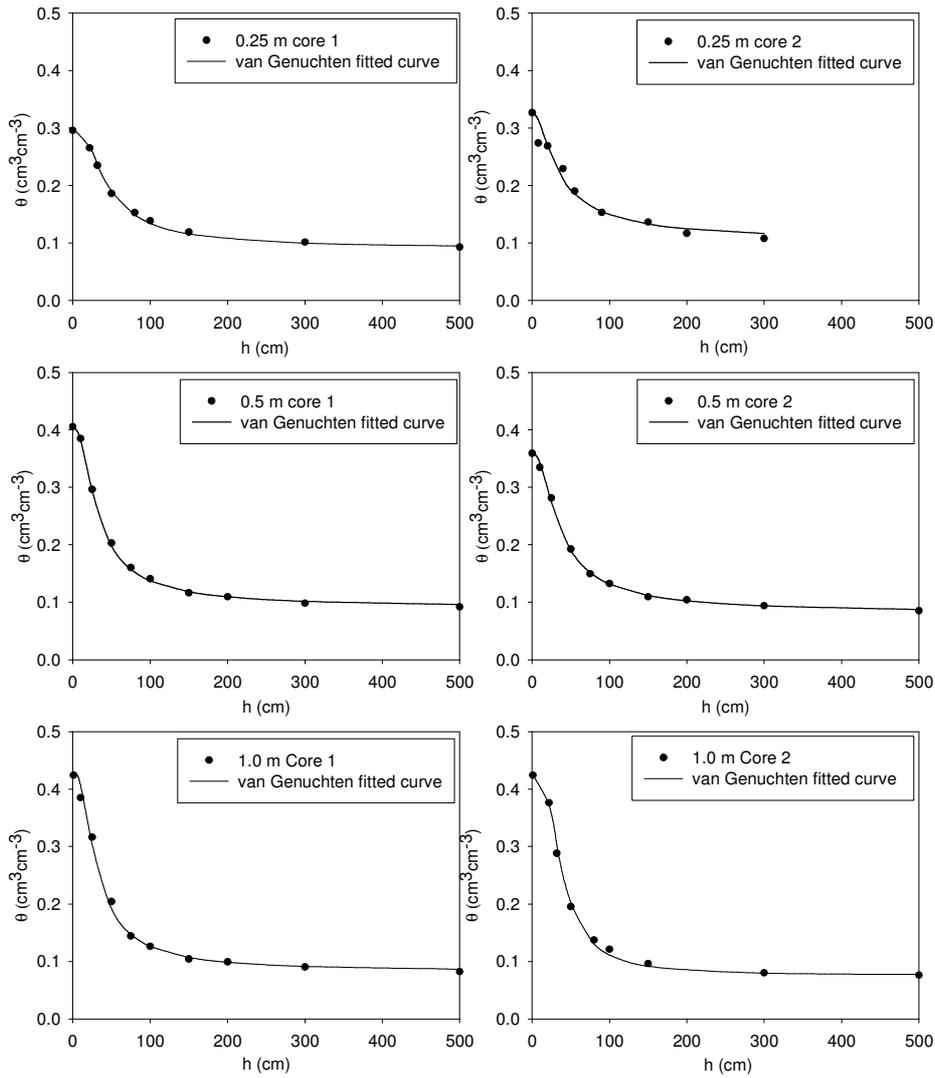
Figure 4.4: AFS soil moisture release curves.
