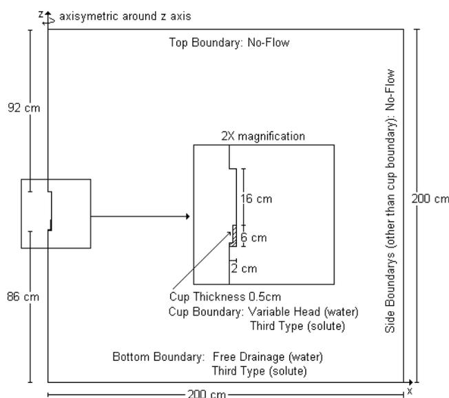
**Figure 2.1:** Axi-symmetric model domain showing the geometry, scale and boundary conditions. The cup boundary has been 2x magnified.
