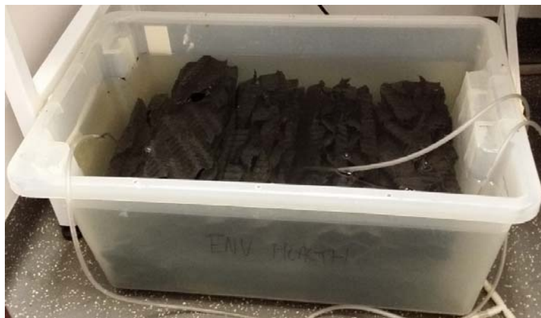
Plate 2.3. Immersing polypropylene media in diluted activated sludge
