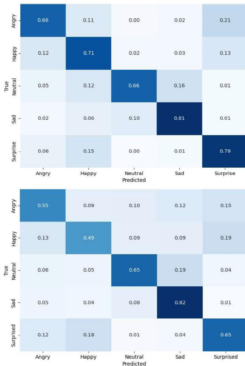
Figure 15. Confusion Matrices for baseline model (top) and the model trained with Sobel-filtered MFCCs (bottom). Horizontal axis represents the predicted emotions while the vertical axis represents the true emotions. Higher average recall is indicated by darker blue.
