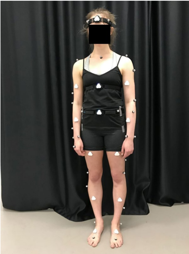
Figure 4-2 Participant with triangular Notch sensors and round reflective Vicon markers in situ
