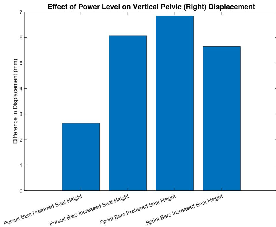
Figure 28 Effect of increasing power level, from submaximal to maximal, on vertical pelvic displacement. Vertical pelvic displacement represents pelvic rocking during pedalling.
