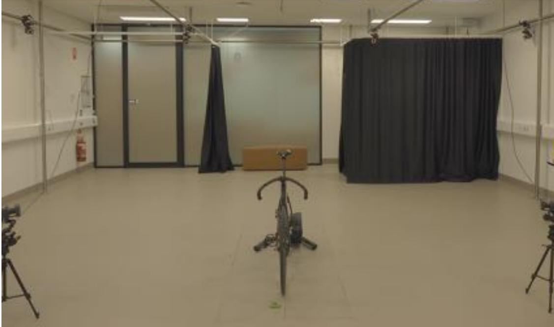
*Figure 13 Location of the cycling ergometer and athletes bicycle used for testing*
