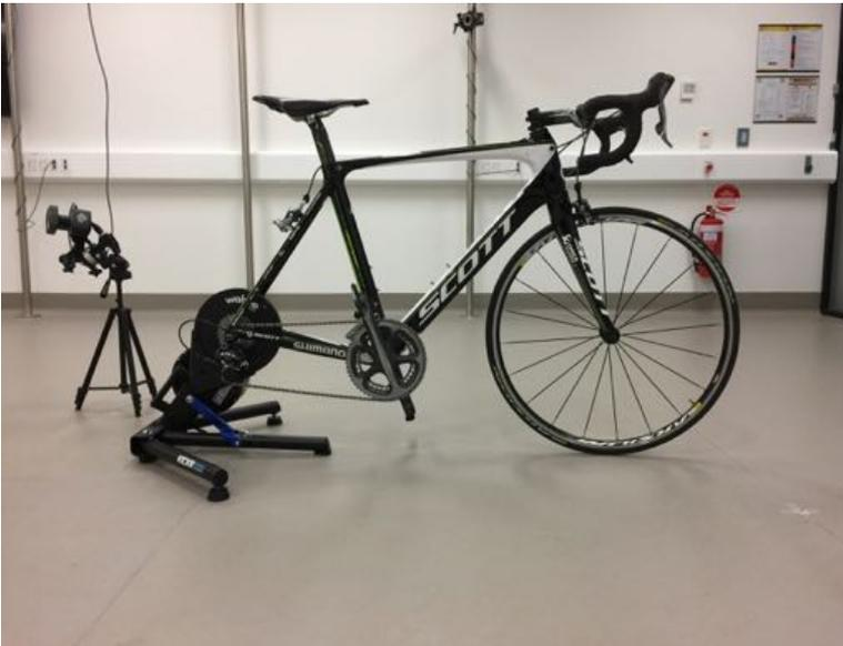
Figure 4 Ergometer Attached to Road Bicycle (Examples only, testing will be done on track bikes with a LeMond Ergometer)
