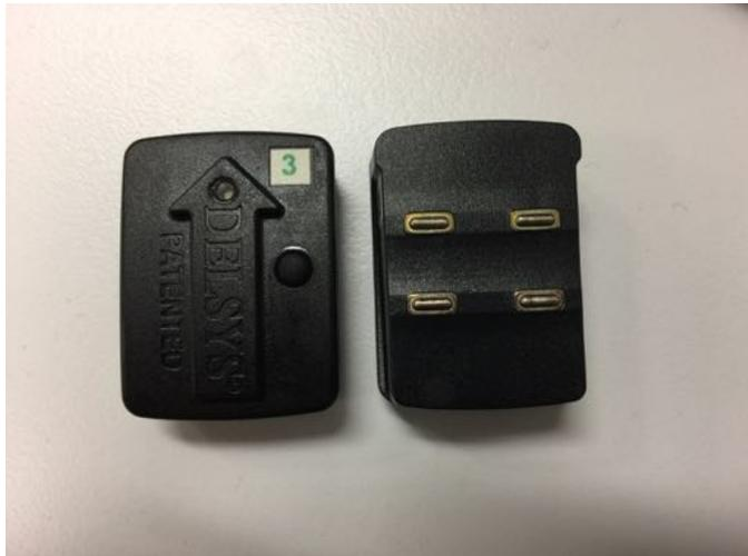
*Figure 7 Example of a Delsys wireless EMG electrode. Arrow on the electrode is to orientate the device with the direction of the muscle fibres.*
