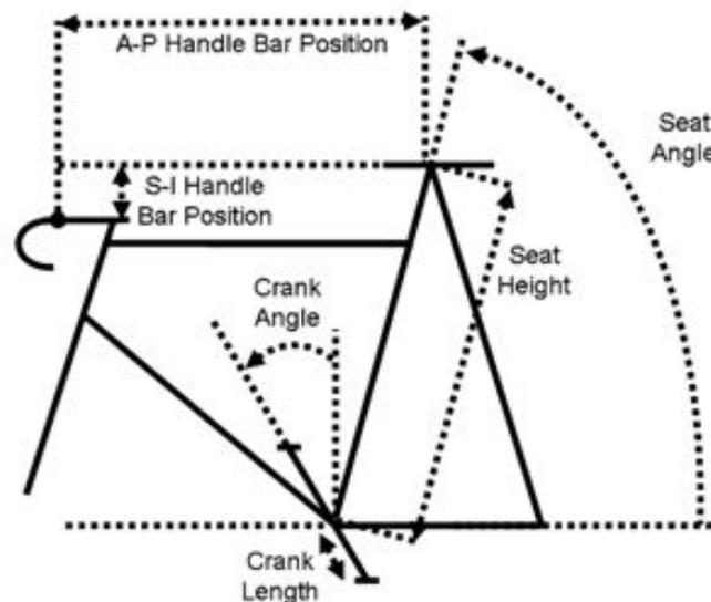
Figure 4 Definitions of bicycle parameters that can be changed [29]
