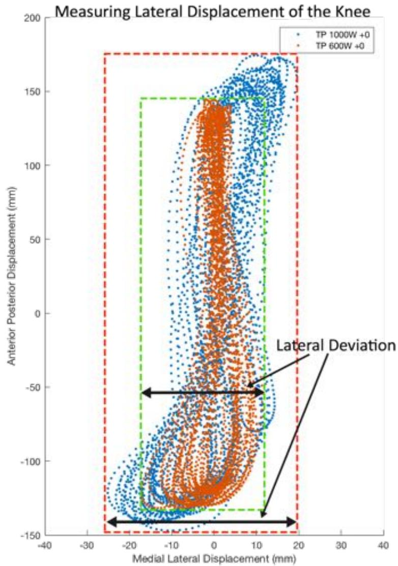
Figure 20 Calculation of the lateral displacement in the transverse plane of the athlete's right knee marker, overlaying two examples of lateral deviation in the same athlete. Plot displays the knee trajectory in the X-Y plane (top view) with positive y-axis showing direction the athlete was facing.
