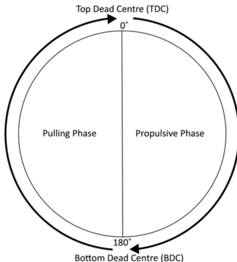
*Figure 2 Crank cycle and main phases of crank cycle during motion analysis*
