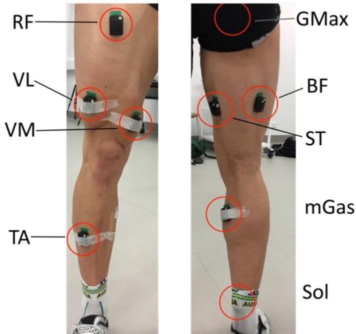
Figure 14 EMG electrode placement during testing. Left side of image is anterior side of the right leg, right side of image is posterior side of the right leg.
