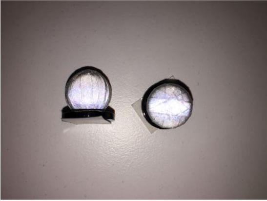
Figure 1 Reflective Motion Capture Marker
