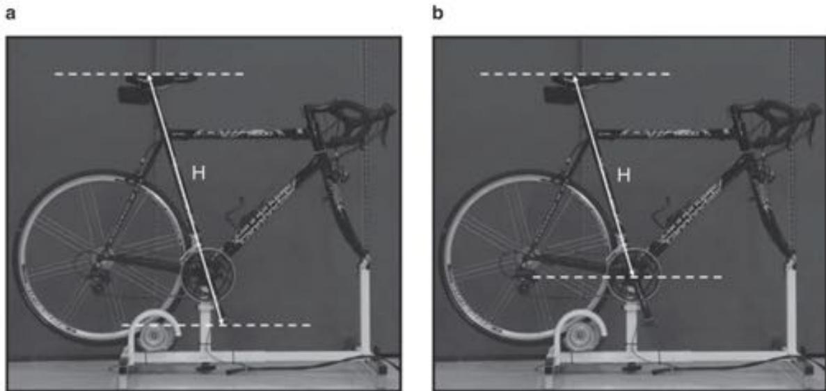
Figure 5 Different ways to measure seat height (a) Hamley and Thomas method of measuring seat height (b) LeMond method of measuring seat height [9]
