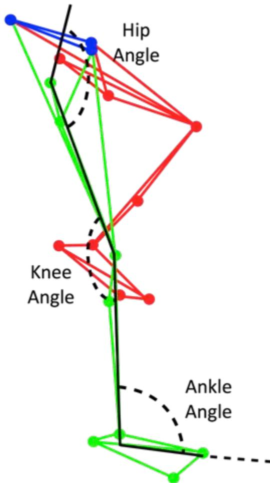
Figure 3 Visual representation of the joint angles present in the sagittal plane of the lower limb. Red lines represent the left leg and green represents the right leg. Joint angles are defined using the right leg in this diagram.
