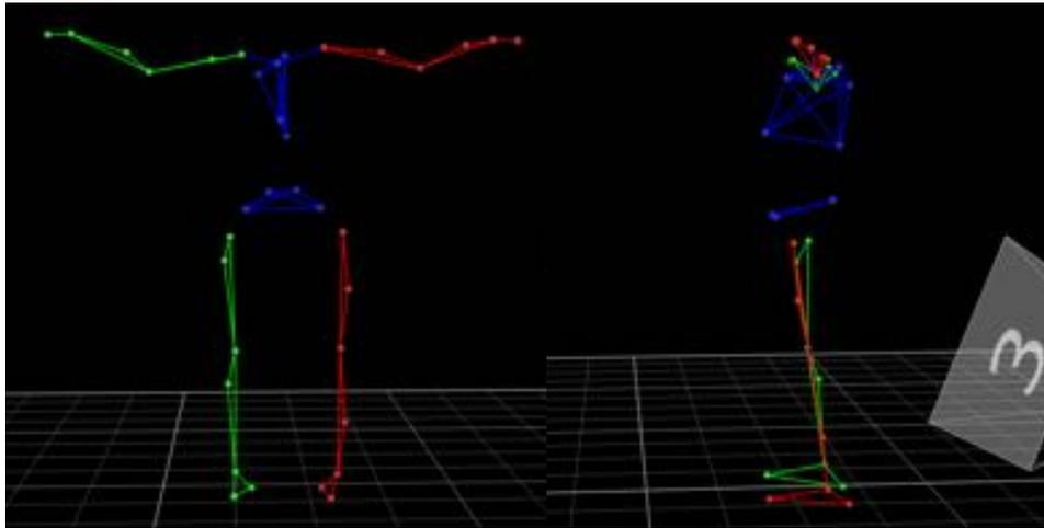
Figure 9 Marker set used in first round of pilot testing. Left side of image shows the anterior view of the T-pose, right side of image shows the left sagittal view of the T-pose.
