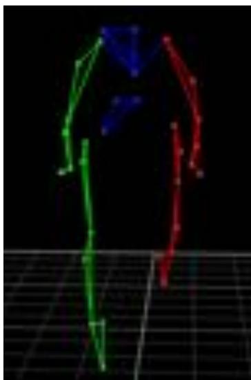
Figure 10 Example of marker loss in pilot testing. Showing that on the left ASIS and sternum marker are missing from the capture. (frontal view)
