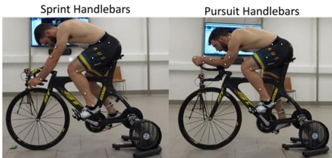
Figure 16 Example of athlete riding sprint handlebars (left) and pursuit handlebars (right).
