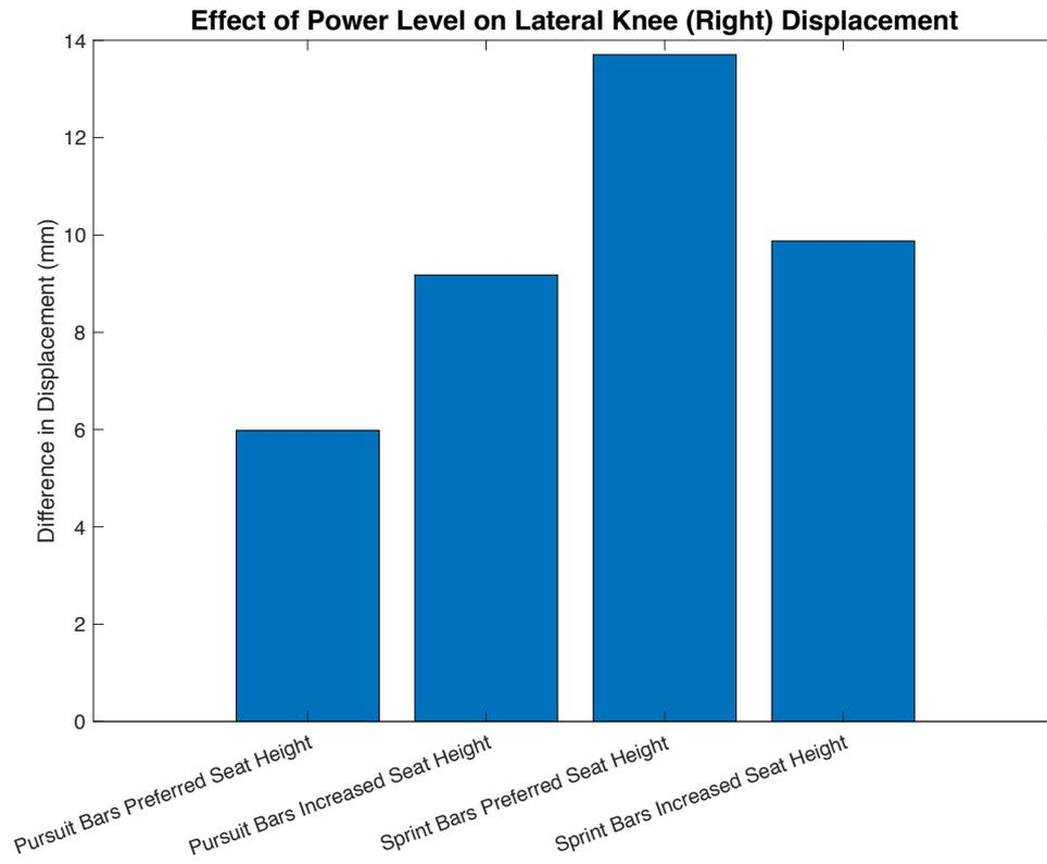
Figure 27 Effect of increasing power level, from submaximal to maximal, on right lateral knee displacement.
