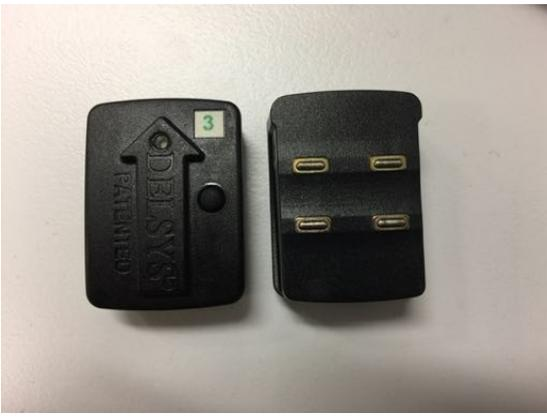
Figure 2 Delsys Wireless EMG Skin Electrodes
