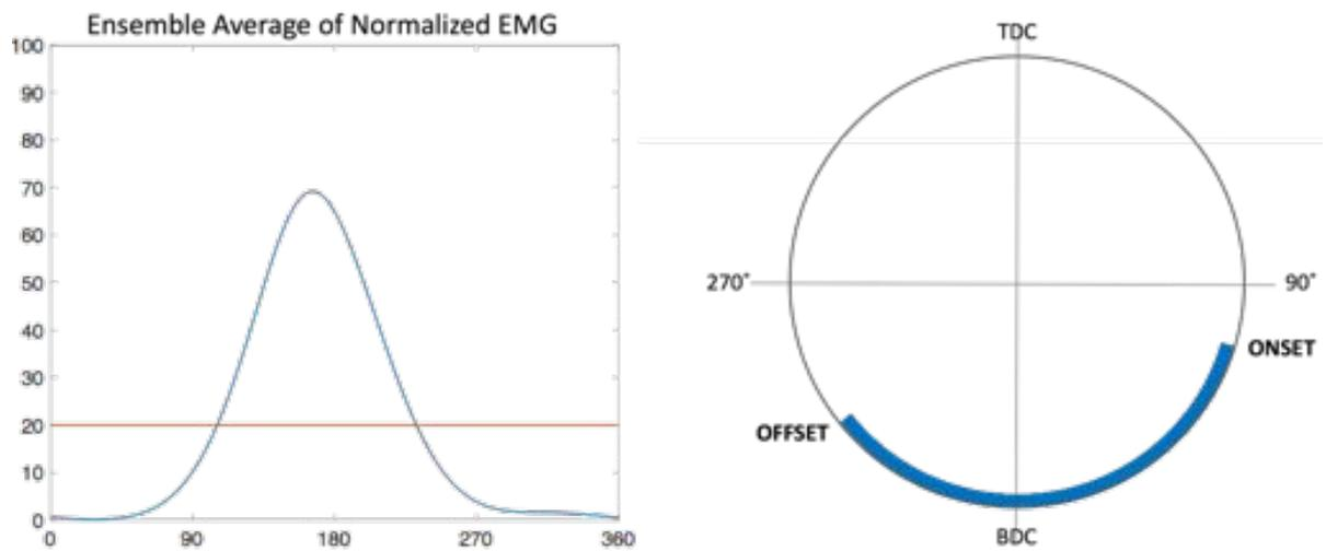
Figure 19 Method of presenting the EMG activation patterns and mapping to the points in the crank cycle. Further graphs will show data in this format to represent the locations of the muscle activation patterns during testing. Threshold of 20% was used to determine the onset and offset.
