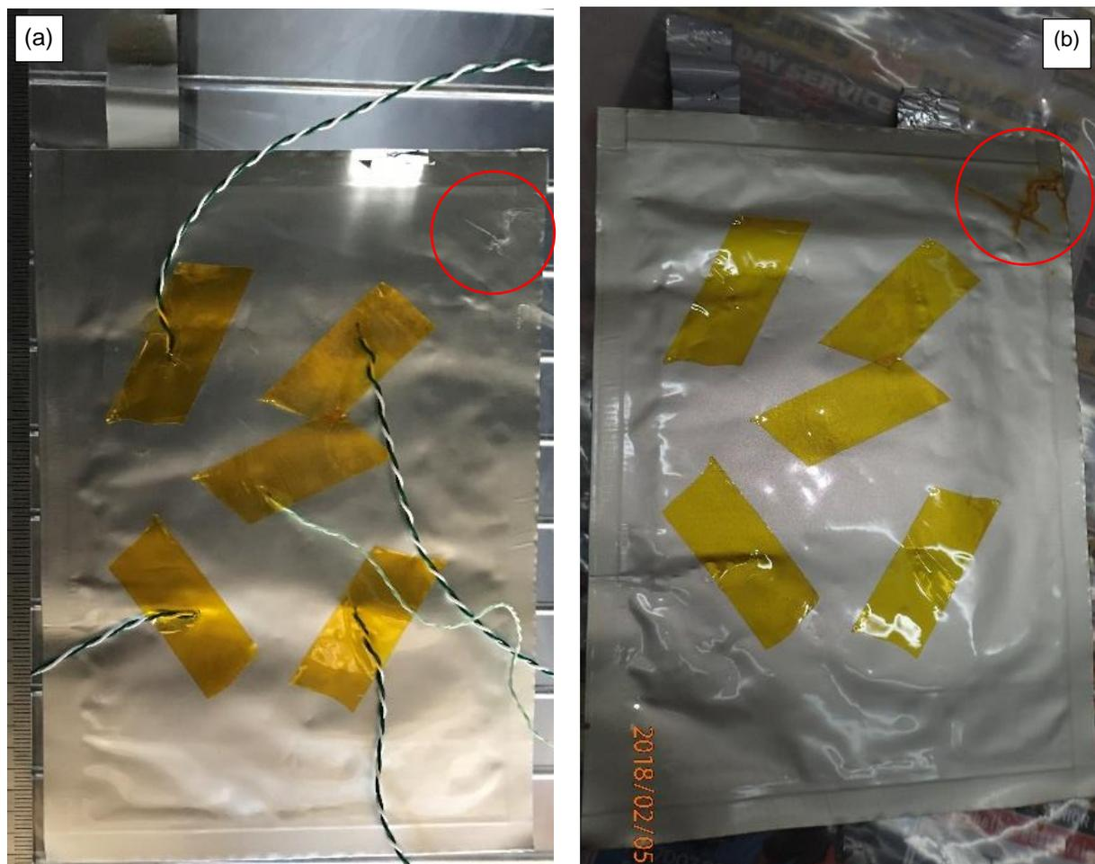
**Figure 6.75** Oven test (a) before and (b) after photos of LFP | P13FSI electrolyte-Celgard 3501 | LTO pouch cell. Discolouration on pouch surface before and after oven testing circled in red.
