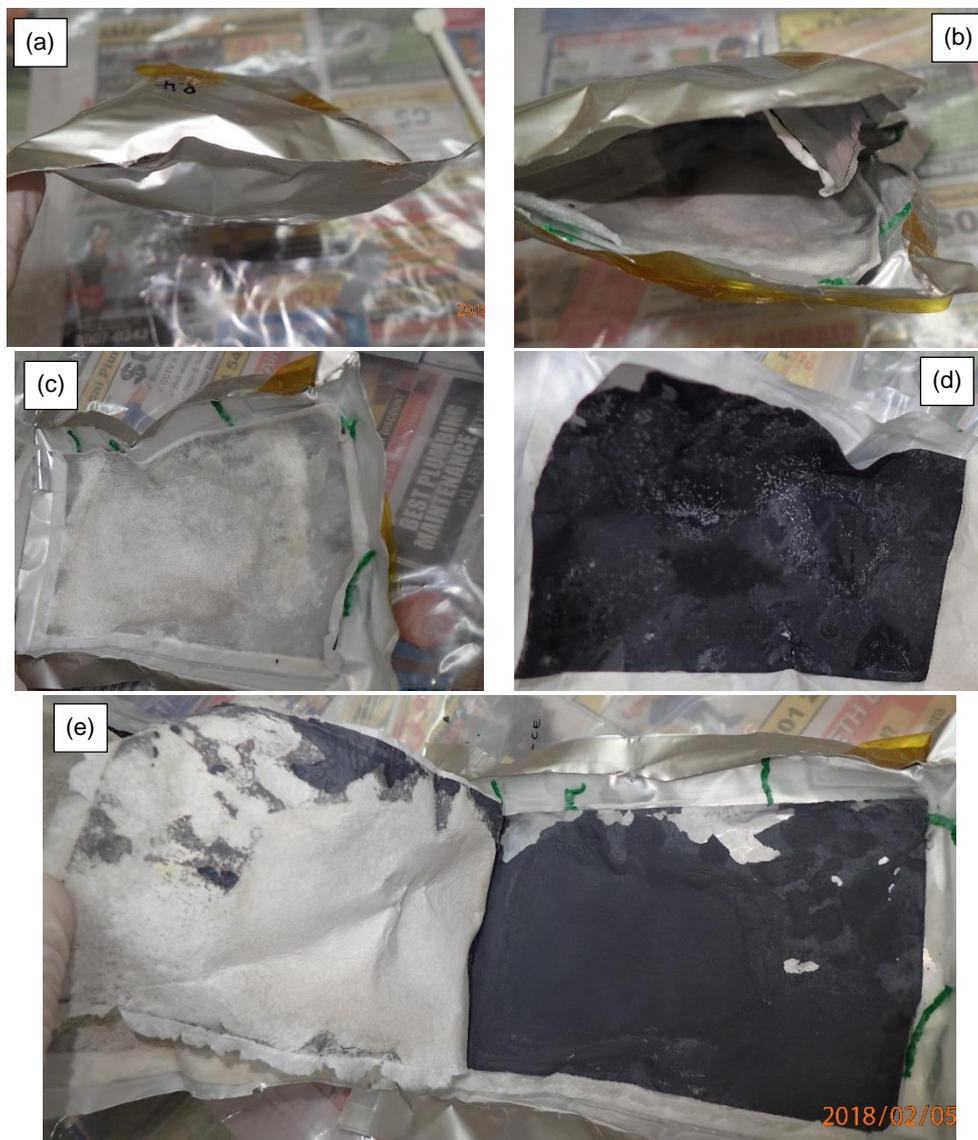
**Figure 6.85** Disassembly photos of a LFP | conventional electrolyte-GF | LTO pouch cell following oven testing.
