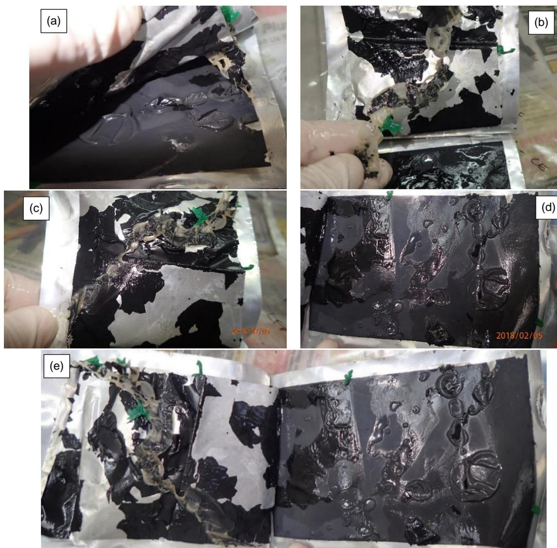
**Figure 6.82** Disassembly photos of a LFP | conventional electrolyte-Celgard 3501 | LTO pouch cell following oven testing.
