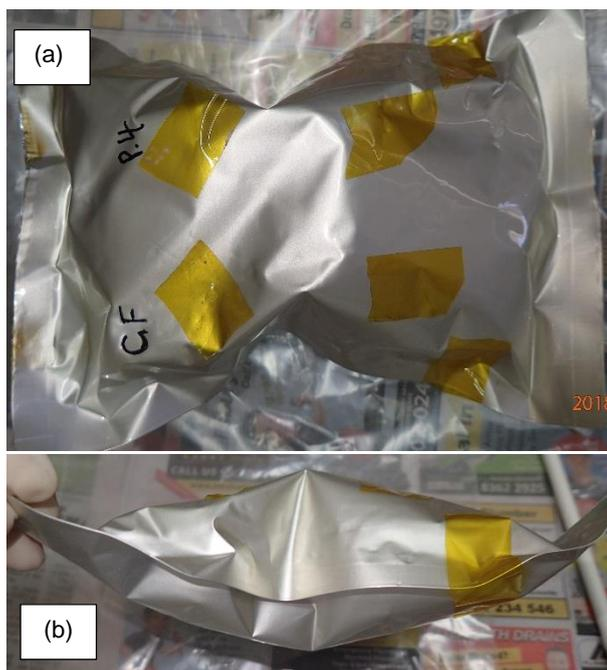
**Figure 6.80** Oven test after photos of LFP | conventional electrolyte-GF | LTO pouch cell, showing severe swelling (a) pouch surface and (b) pouch side.
