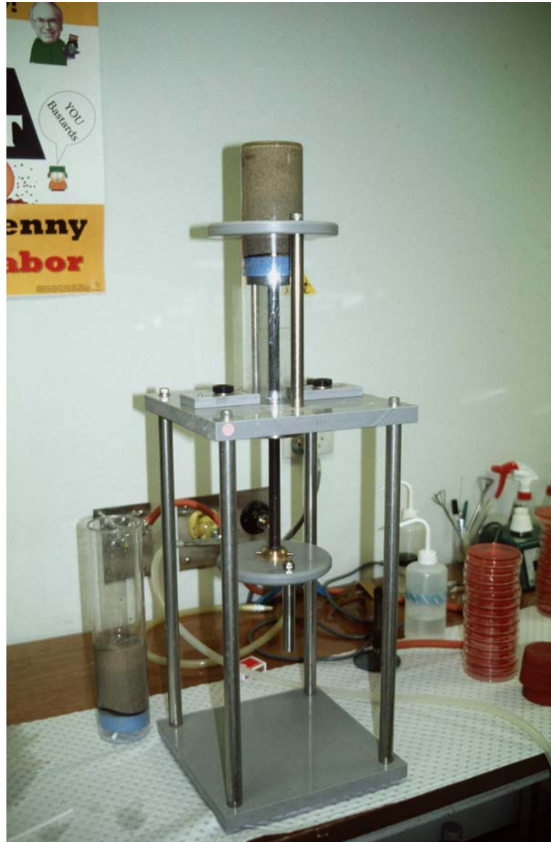
Plate 2.5 Coring device used to extrude sediment at controlled intervals.
