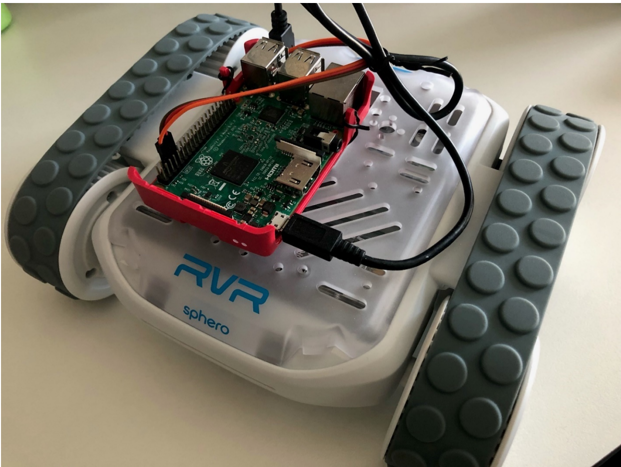
Fig. 5. The control target: Sphero RVR with Raspberry Pi
