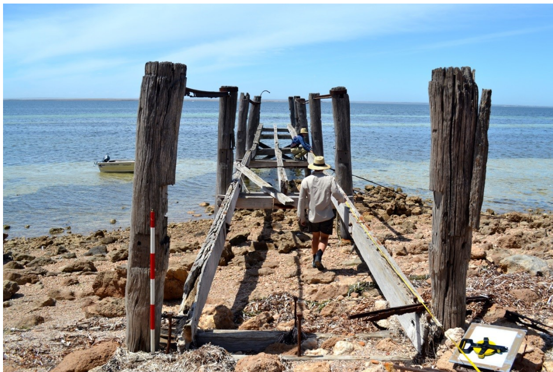
Figure 17 C. Pasch and K. Bennett establishing a baseline for baseline-offset recording of the Little Jetty, facing east (photograph by J. McKinnon 26/2/13).
