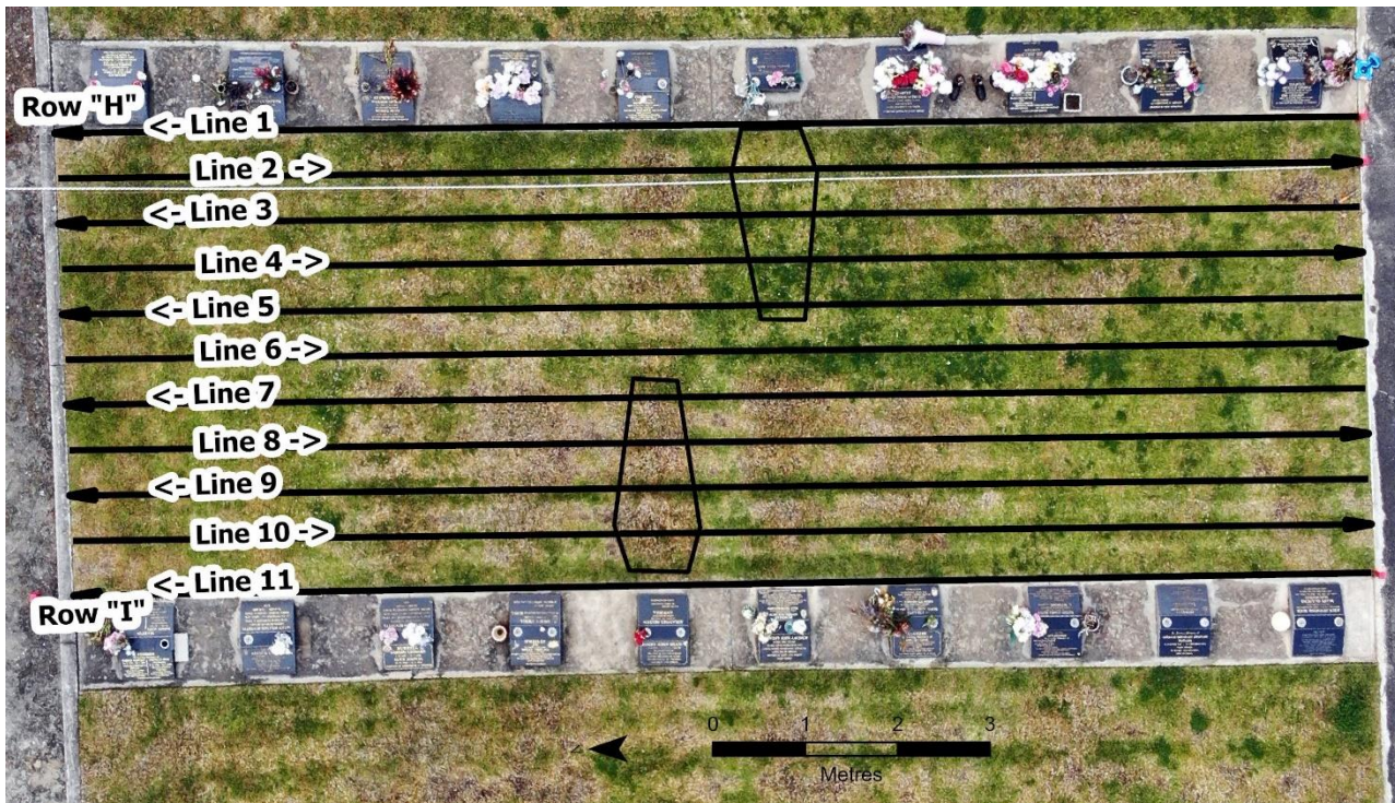
Figure 3.4.1: Rows H and I, Keith Cemetery. The GPR lines are shown, and as the data is collected in a "zigzag" method, every second line is in the opposite direction. The outlines of two graves are shown to illustrate that for Row H, lines 2,3 & 4 are over the widest point of the coffin, i.e. the shoulder and torso. The ERT line is between line 2 and line 3 in Row H.
