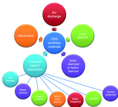
Figure 1. 8 Different methods used to prepare CNTs. This figure has been copied from reference 28.
