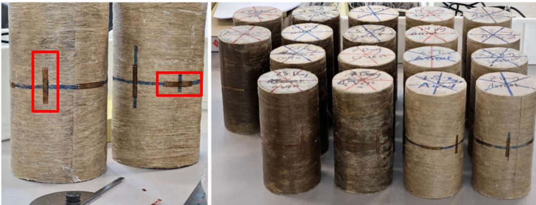
Figure 4: Strain Gauges attached to the samples (left); Sample ready for testing (Right).
