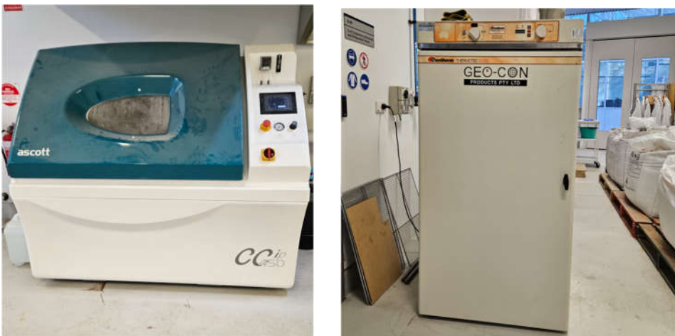
Figure 3: Saltwater spray apparatus (left) and oven (right) utilized for the project.
