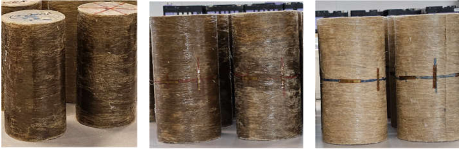
Figure 6: Control samples (left), samples exposed to high heat (middle) and salt spray (right).
