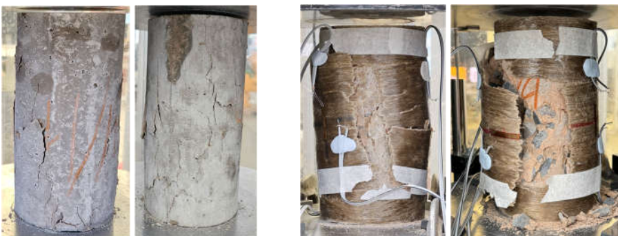
Figure 7: Failure pattern observed in plain concrete samples (left) and FRP-wrapped samples (right).
