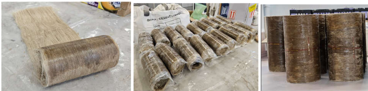
Figure 2: Confining the concrete sample with composite (Left), Samples confined with composites (Middle), and confined samples after the curing process (Right).
