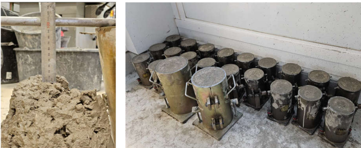
Figure 1: Slump test on concrete mix (Left) and concrete samples left for setting (Right).
