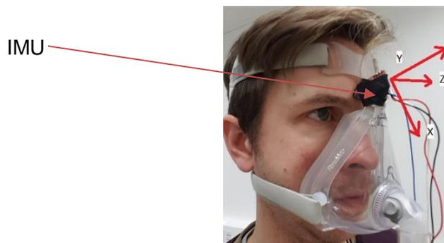
Figure 5-12 - The prototype PAP mask with the IMU attached and the gyroscope axes labelled
