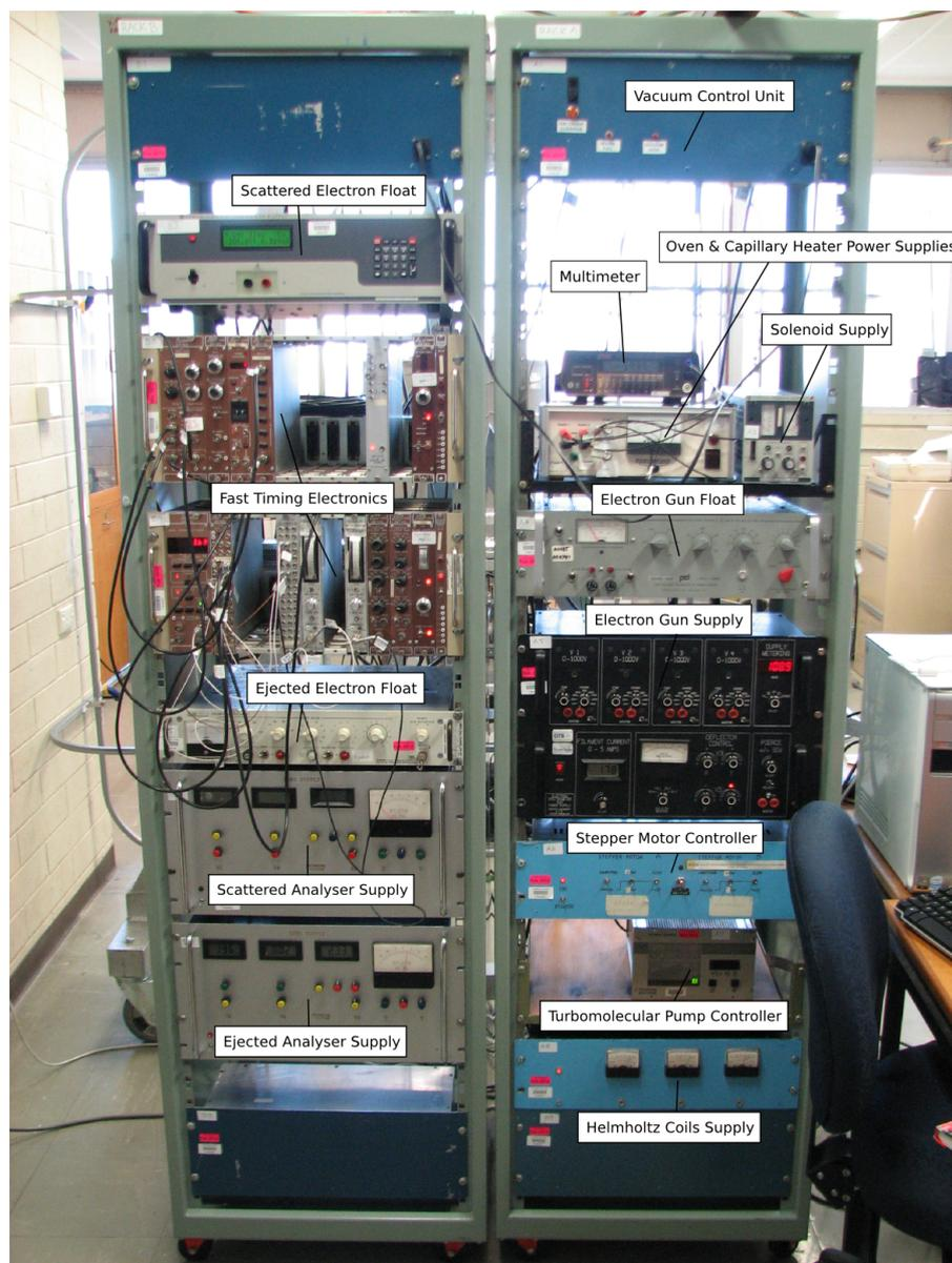
Figure 3.8: Photograph of the control racks, with the various important elements labelled as appropriate.
